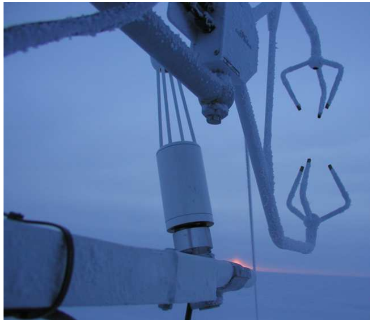
Figure 3.6: The eddy correlation system on the heat budget tower. CSAT3 (sonic anemometer) and LI7500 (CO 2 and H 2 O gas analyzer).
