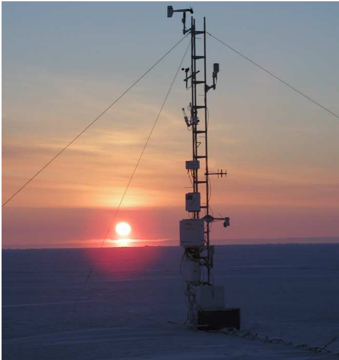
Figure 3.5: The 5m heat budget tower south of Takatuk.
