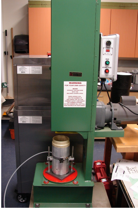
FIGURE 3.9: Automated Impact Compactor for Soil Samples
