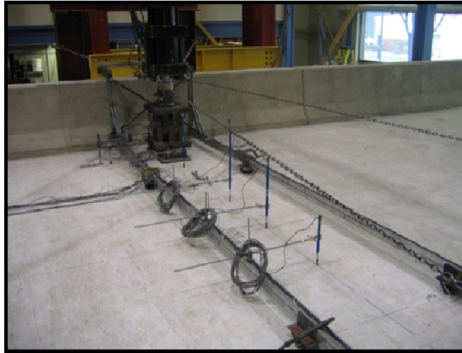
Figure 3-20: Photograph illustrating the LVDT supporting apparatus used to measure deflections of the cantilever and internal panel relative to the girders
