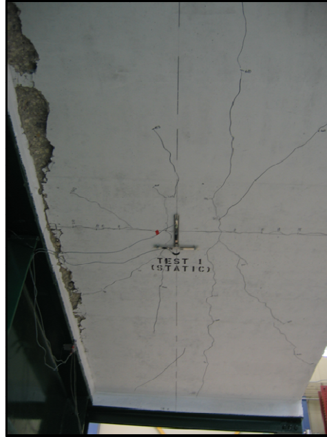
Figure 3-27(a): Photograph showing pi gauge locations on the underside of the cantilever slab overhand under the loading plate (typical all test locations)
