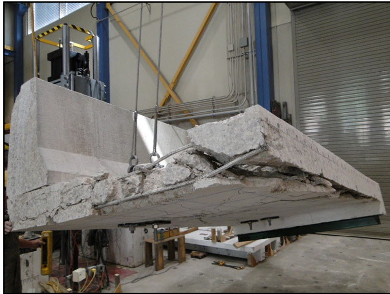
Figure 4-71: Photograph taken during demolition illustrating diagonal shear cracks and punch cone representative of punching shear failure for the cantilever with steel reinforcement subjected to a fatigue cyclic load
