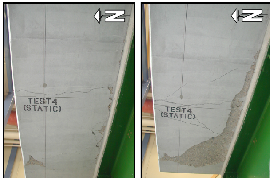
Figure 2-24(a): Top view of semi-circular punching type failure for the cantilever section with top transverse steel reinforcement subjected to static monotonic loading (Klowak, 2007)
