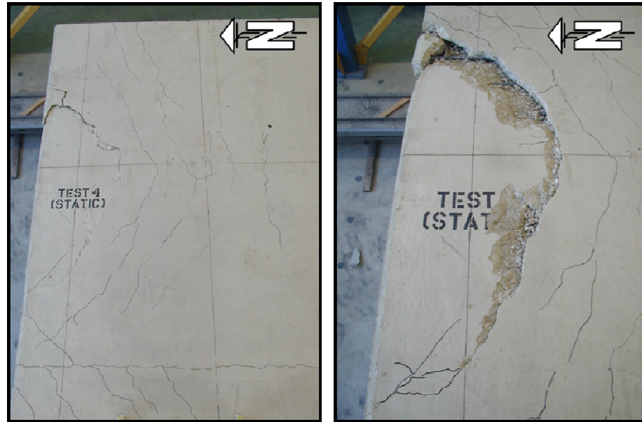
Figure 2-24(a): Top view of semi-circular punching type failure for the cantilever section with top transverse steel reinforcement subjected to static monotonic loading (Klowak, 2007)
