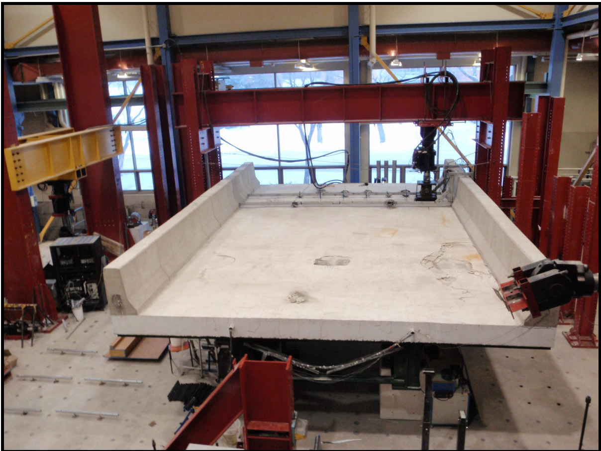
Figure 3-17: Photograph of test set-up for static and fatigue destructive testing of cantilevers
