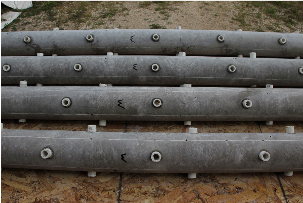
Figure 38: CFPTs After Testing @ Mid-Span (ordered #1 closest to # 4 farthest)
