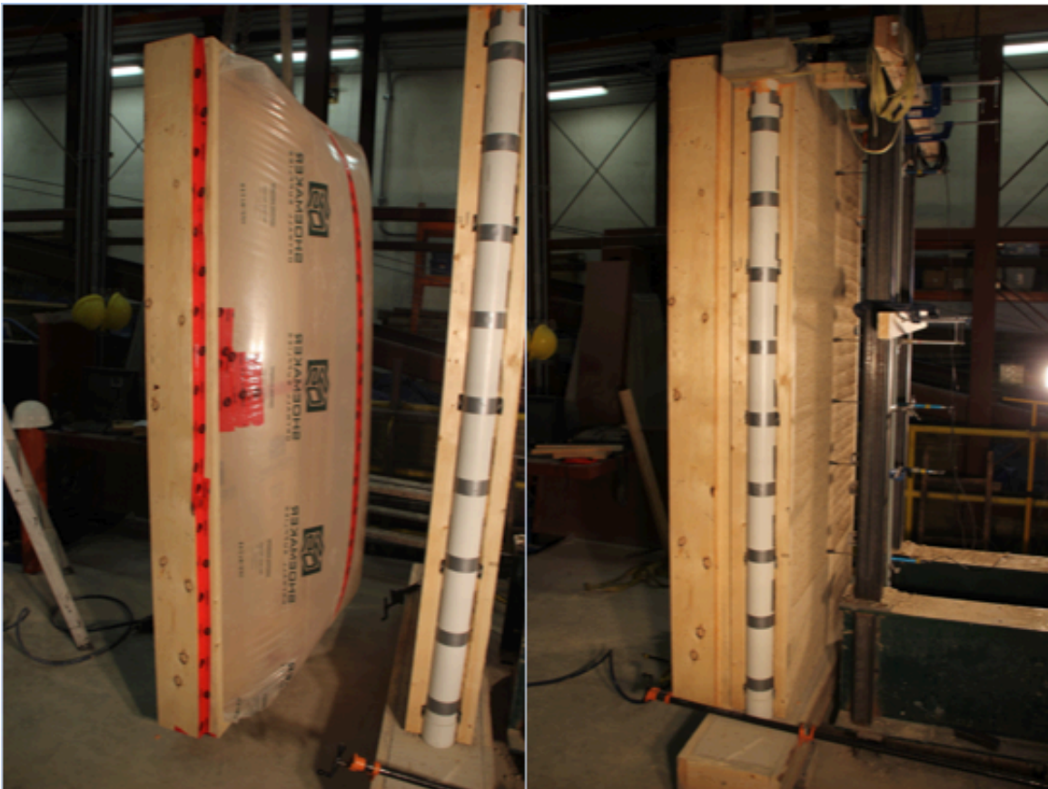
Figure 25: Airbag Assembly Pressurized (L) and Secured to Wall System (R)
