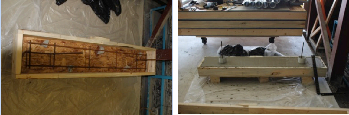
Figure 15: Empty Concrete Footing (L) & Poured With 102 mm (4") PVC Unions (R)
