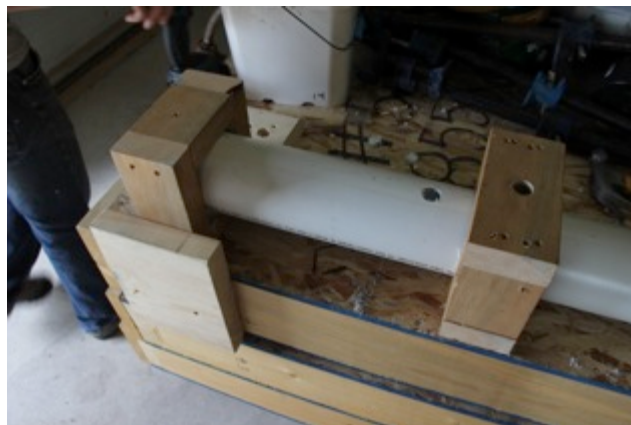
Figure 4: Jig for Aligning and Drilling Holes in PVC Tube
