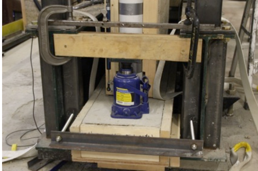
Figure 22: Cyclic Loading Footing Restraint and Linear Pot
