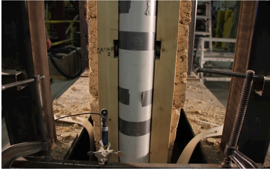
Figure 42: Racking Wall 1 - Compacted Adobe Separation @ 1800 mm (70") From Top
