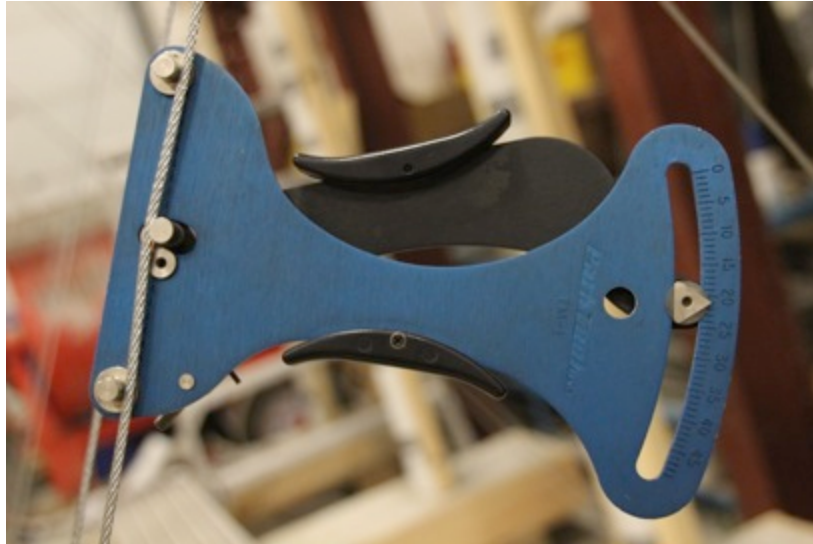
Figure 14: Tensioning Aircraft Cable with Bicycle Spoke Tension Meter
