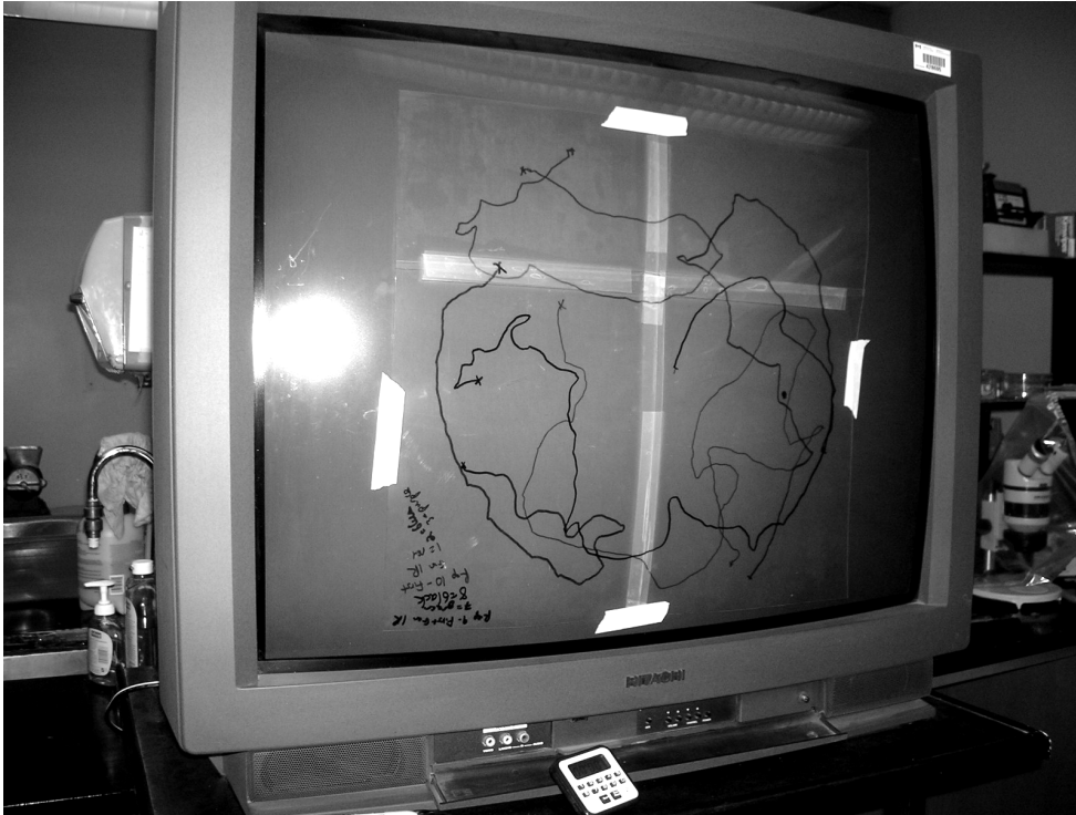
Figure 5.13. Setup used to measure rate of movement. A sheet of acetate was placed over a TV monitor and a timer (bottom middle) was used to time one minute.
