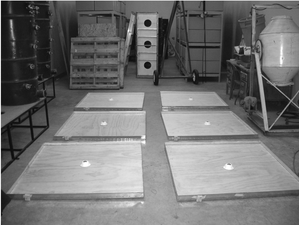
Figure 5.8. The arena experiment. Two hundred beetles of various strains and species (mill or laboratory/ Tribolium confusum or Tribolium castaneum ) were placed in an arena with a monitoring trap for 24 hours, in the dark. The number of beetles in and beneath the trap was then recorded.
