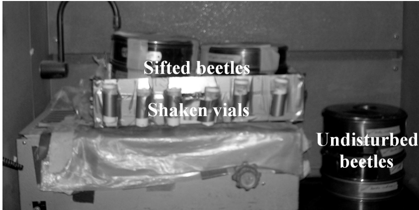
Figure 3.1. Setup for shaking and sieving disturbances. For the shaking condition, beetles were placed in each vial and vials were attached to an automatic shaker. For the sieving condition, beetles were placed on 425 \mu\text{m} sieves which were put in the automatic shaker. Undisturbed beetles for the sieving condition were placed on 150 \mu\text{m} sieves.
