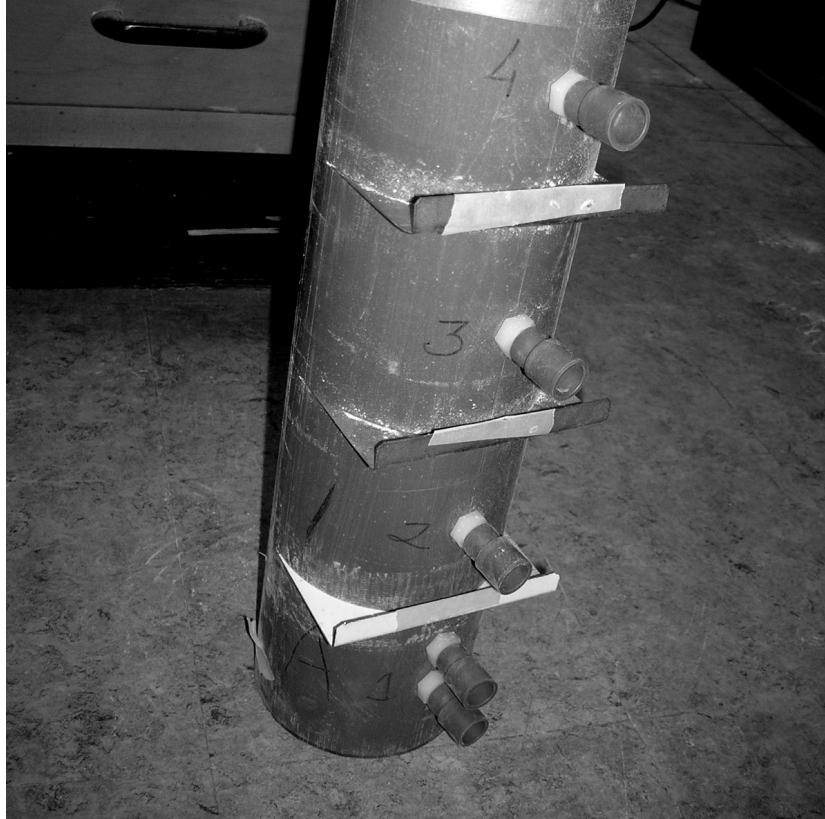
Figure 5.15. Tubes used to measure beetle distribution throughout a 36cm height of flour. 200 Tribolium beetles of a known species and strain were placed on the top of the flour height and left in the dark for 24 hours.
