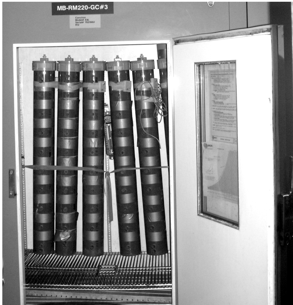
Figure 5.16. Tubes secured inside an incubator. Tubes were left undisturbed and in the dark for 24 hours.
