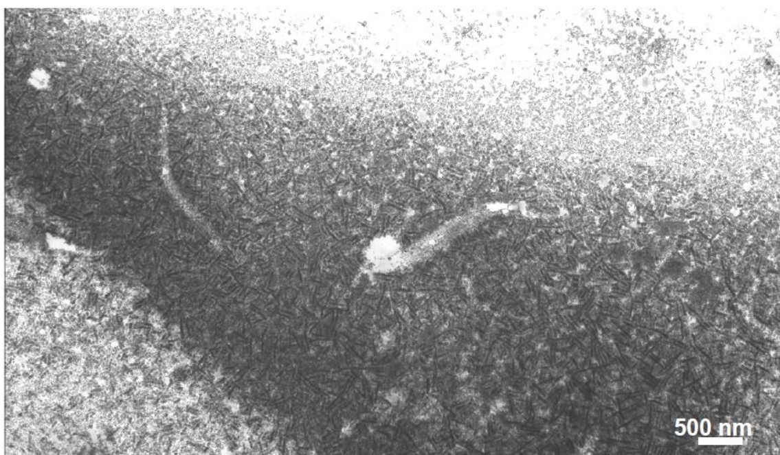
Figure 3.3. TEM image showing the large-area self-assembly of the DLC-GNRs. Several GNR ribbons extend over several hundred nanometers.
