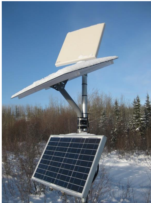
Figure 4.23: Plastic awning added to shield solar panel from snow. December 1, 2012.
