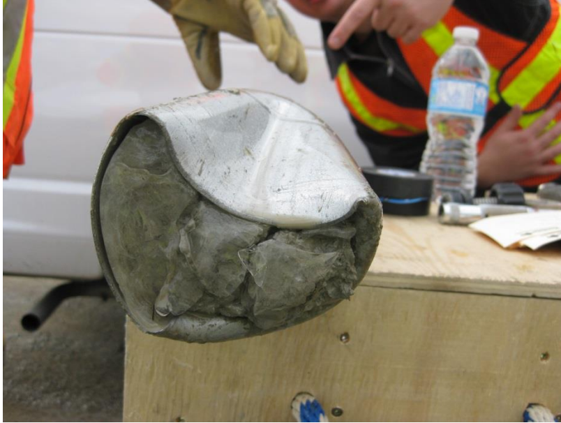
Figure 3.10: Damaged four inch Shelby tube obtained from the shoulder. September 11, 2012.
