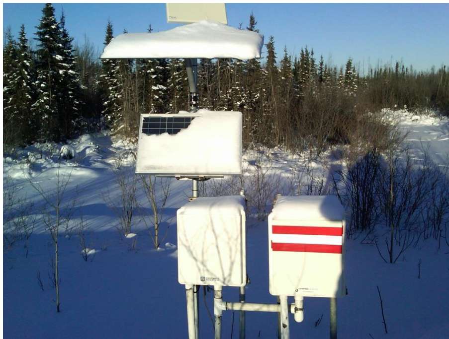
Figure 4.24: Snow cover issues persisted after plastic awning added contributed to loss of batteries. January 17, 2013.
