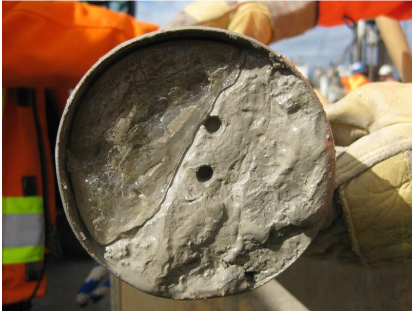
Figure 3.5: Frozen ground and ice encountered at the shoulder. September 11, 2012.
