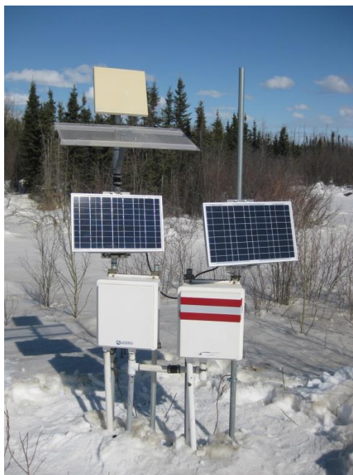
Figure 4.25: Second solar panel added and both solar panels tilted to a nearly vertical angle. March 27, 2013
