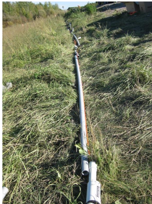
Figure 4.6: Multilevel Vibrating Wire Piezometer prior to gluing the connections and installing vertically at the centreline. September, 14, 2012.
