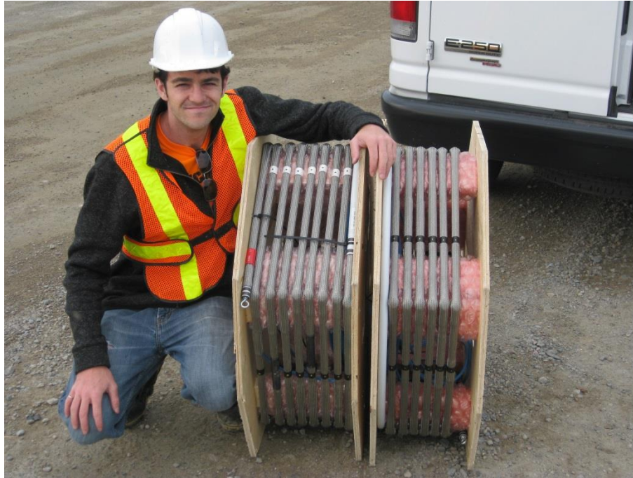
Figure 4.5: ShapeAccelArrays on their factory issued bundles. The white tape with the black dots indicates the direction of the x-axis. September 10, 2012.
