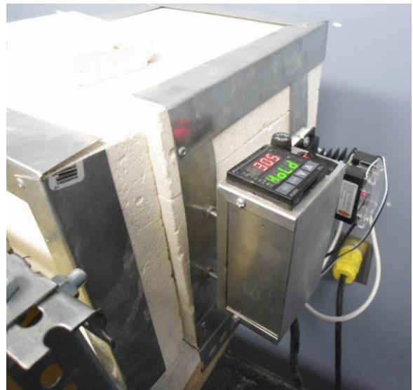
Fig. 24 Furnace and high temperature test chamber attachment to DIHPB showing interior and control box
