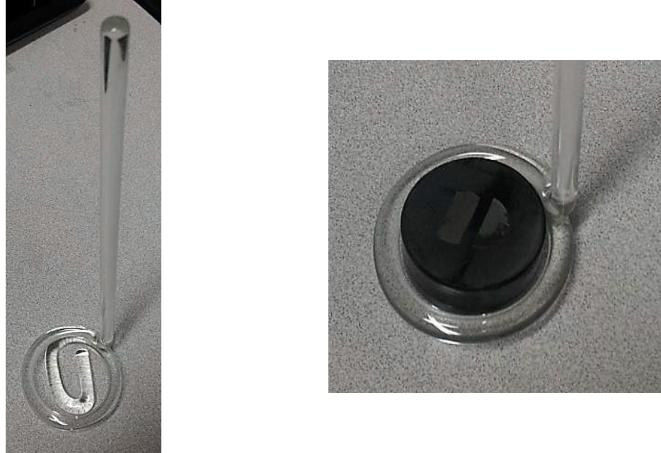
Fig. 32 Glass holder for Bakelite mounted specimens during etching
