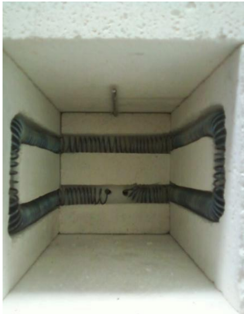
Fig. 24 Furnace and high temperature test chamber attachment to DIHPB showing interior and control box
