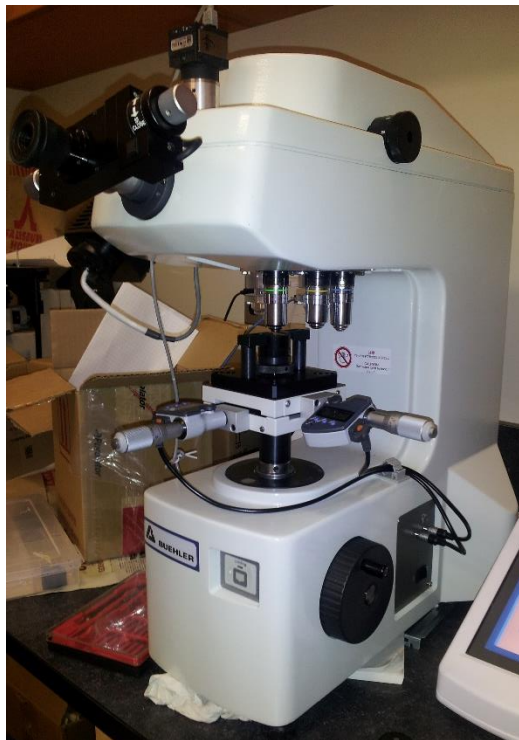
Fig. 69 Buehler Micromet 5100 Series micro-indentation machine for measuring Vickers hardness of specimens (image taken by this author)
