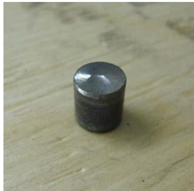
Fig. 28 AISI 4340 Steel Specimen prior to heat treatment
