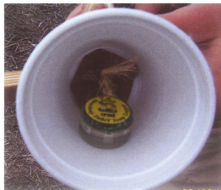
Figure 3.3.1 Air temperature data collection mode. A StowAway Tidbit Temp Logger by Onset suspended from within a Styrofoam™ cup (A. S-Hermann 2006).
