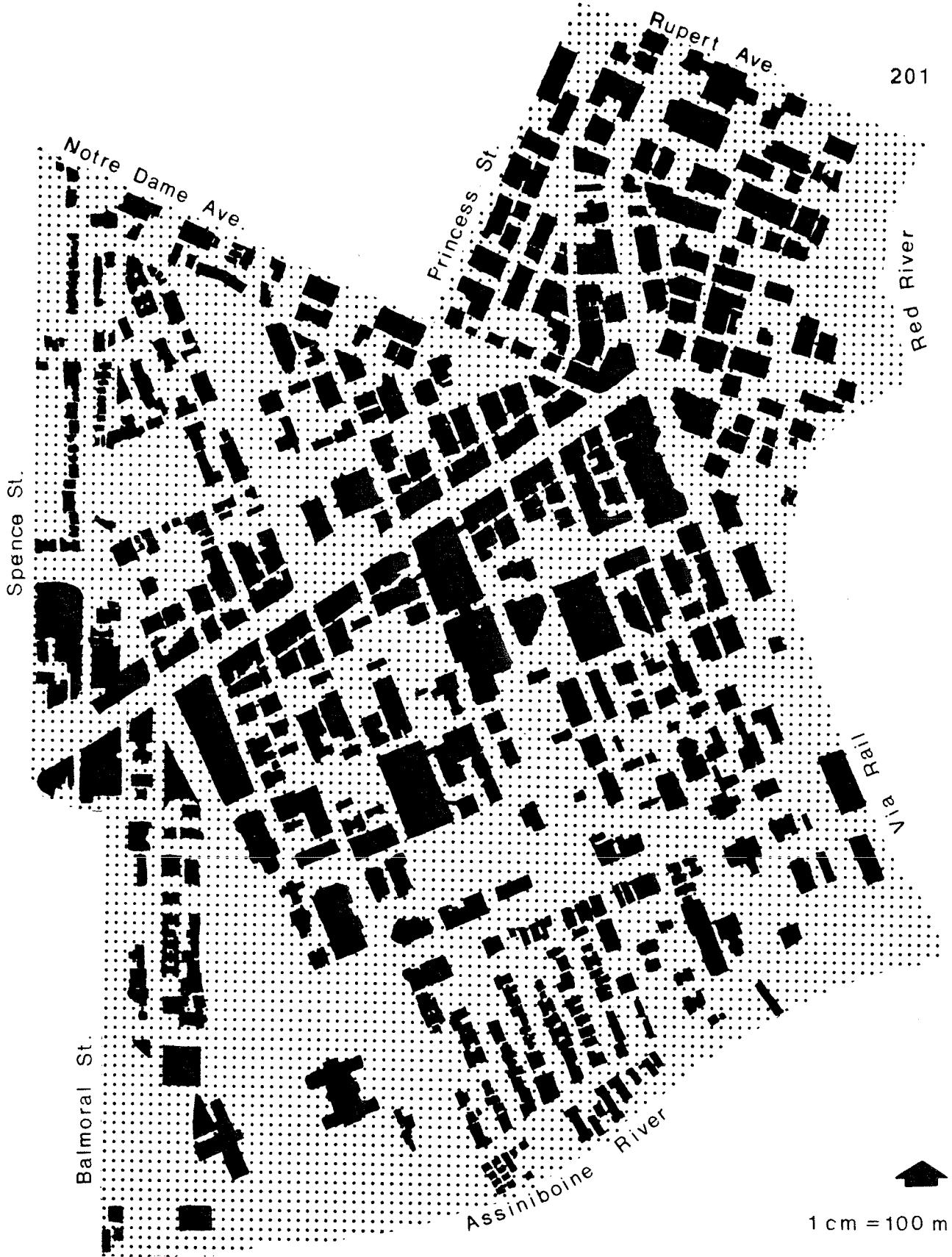
Figure 118: Roof Space in Downtown Winnipeg (The total roof space equals about 23% of the total area.)
