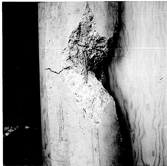
Column 1 A p Showing failure due to eccentric load
