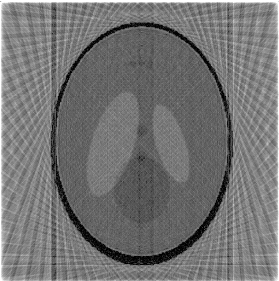
Figure 27: FBP reconstruction of Shepp & Logan 512x512 from 37 angles with manual window and level adjustment.
