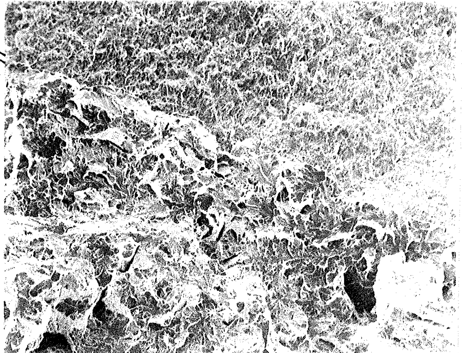
Figure 4.26 Scanning electron micrographs from two WLCT specimens showing the stretch zone during impact tests. (100 X)
