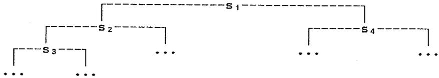
the dashed line denotes paths through several possible levels. An address formed at any particular point is made relative to the closest containing reference point (i.e.  $s_1$ ,  $s_2$ ,  $s_3$ , or  $s_4$ ).
