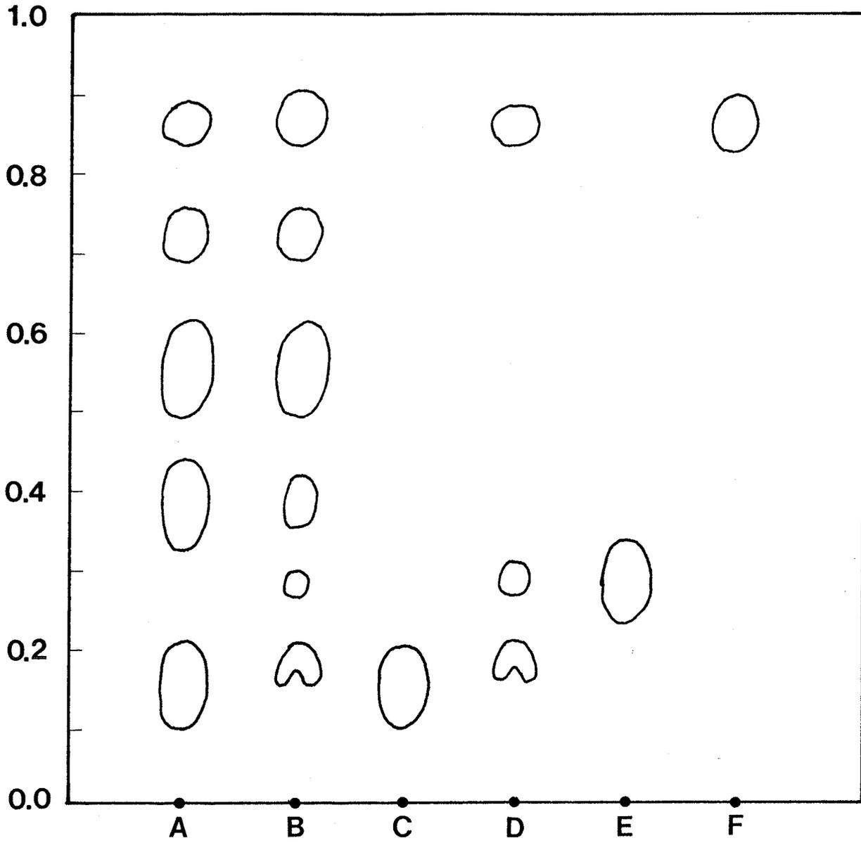
Figure 11. Activated Carbon Treated Freeze-Dried MCE Rechromatographed with Sephadex G25.
