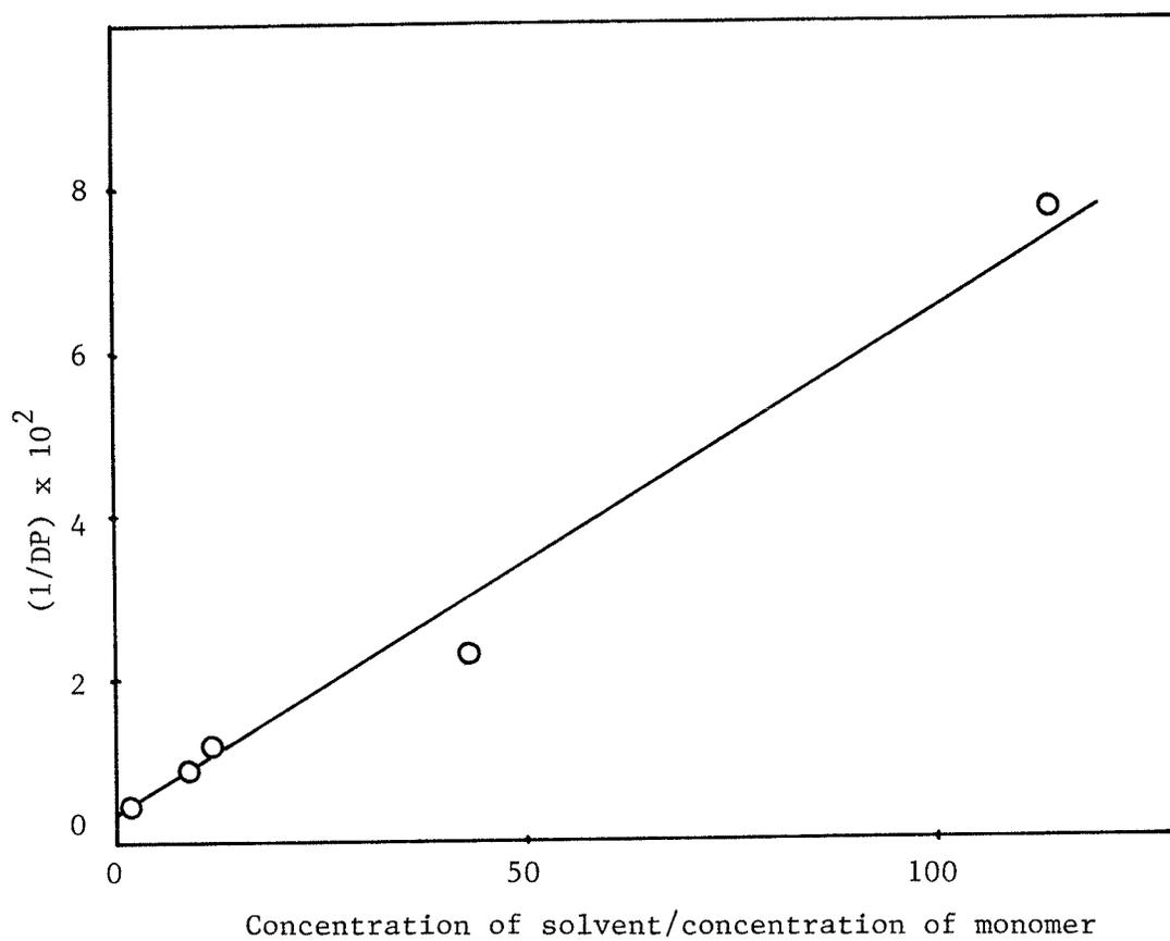
Figure 2: DP of PVAc as a function of monomer concentration in methanol
