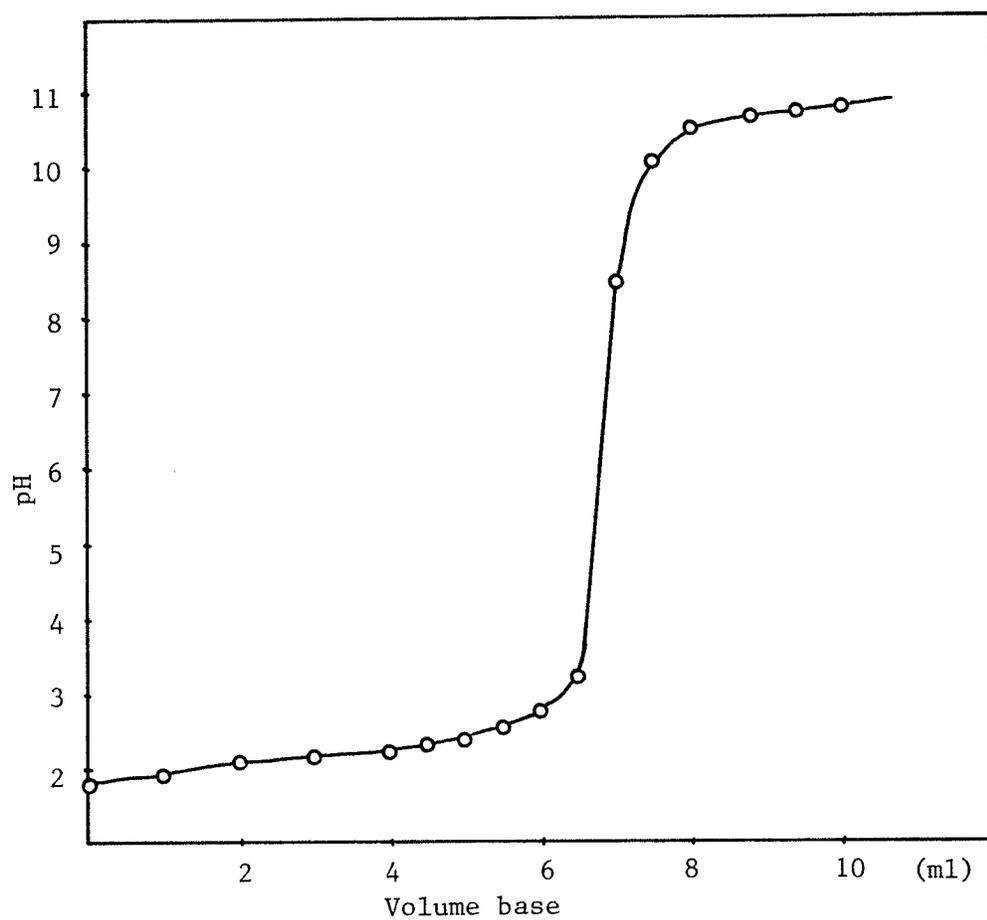
Figure 15: Titration of PVA-CO<sub>2</sub>H with sodium hydroxide
