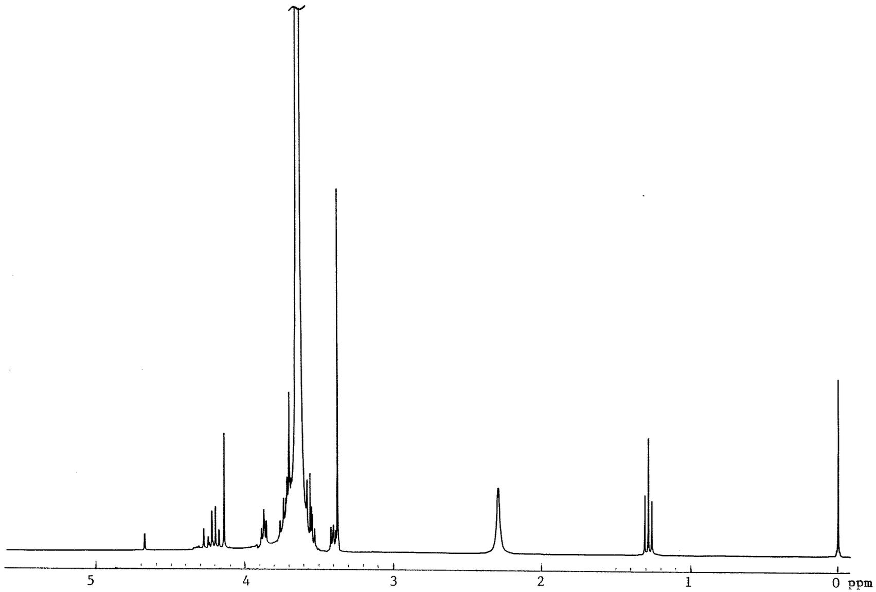
Figure 8:  $^1\text{H}$  NMR of PEG-O-CH<sub>2</sub>CO<sub>2</sub>H prepared with Na/naphthalene.
