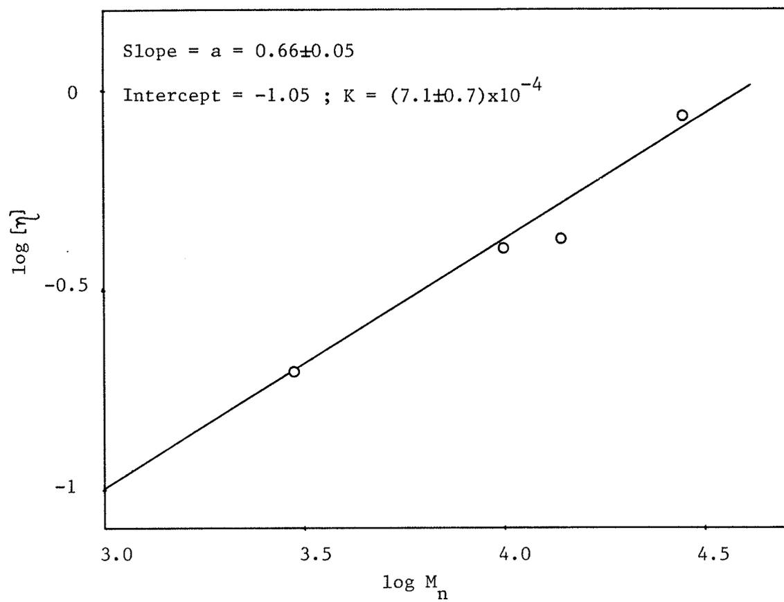
Figure 13: Determinations of constants  $a$  and  $K$  in Mark-Houwink's equation
