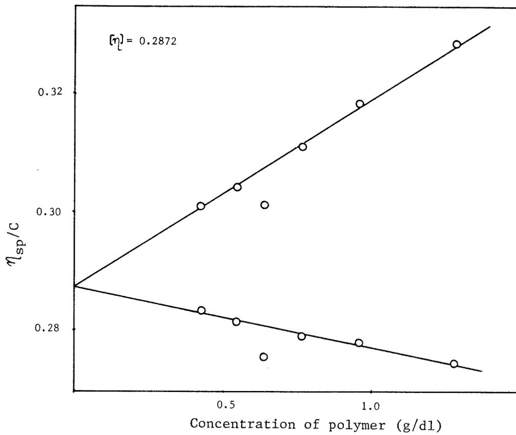
Figure 14: Determination of the intrinsic viscosity of PVA-OH
