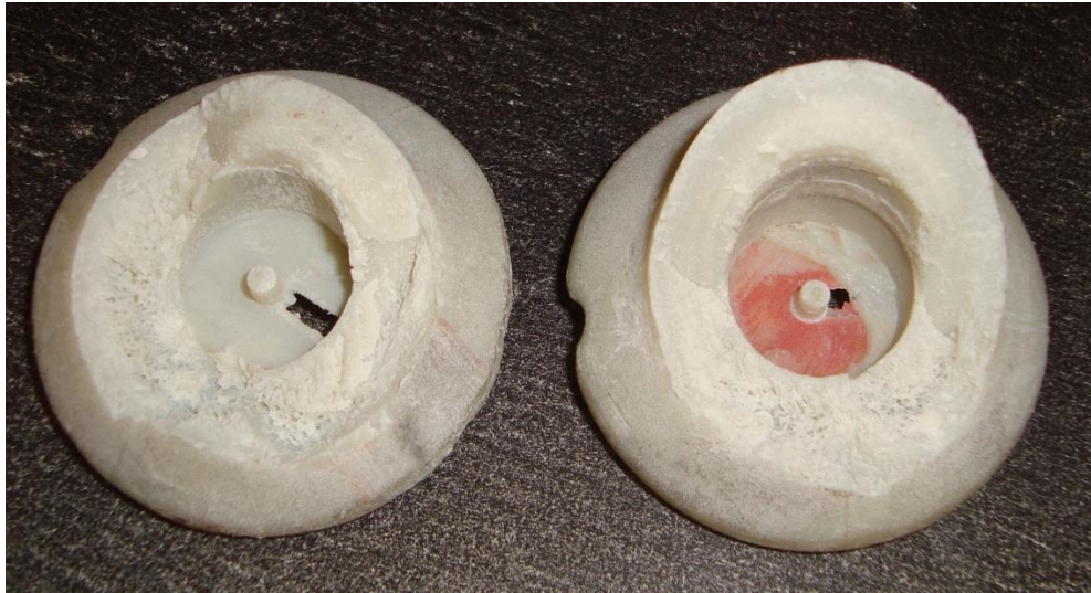
Figure 5.19: Typical bearing failure of anchorage heads in Specimens I-H-D and I-H-S
