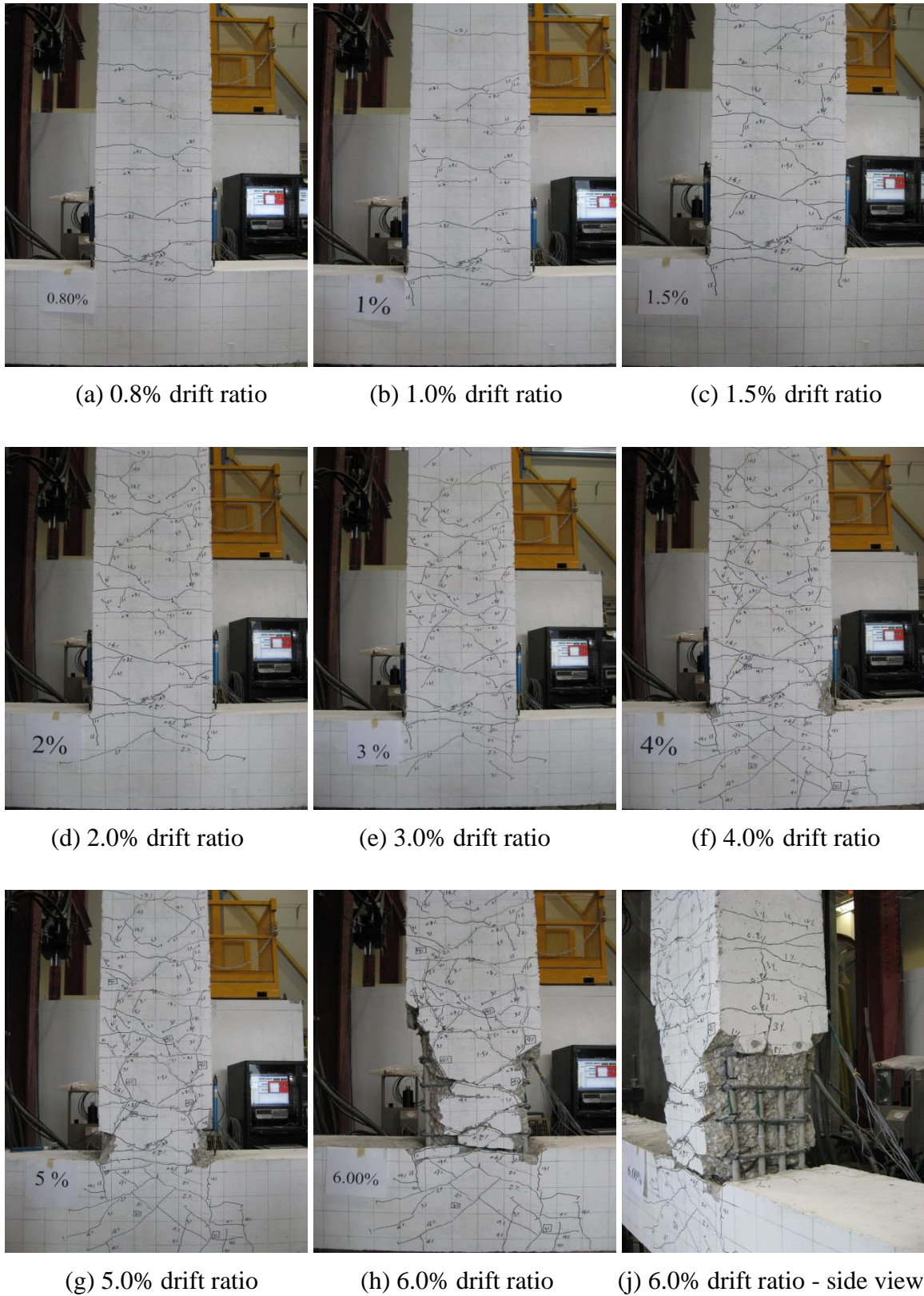
Figure 5.5: Cracking progression of Specimen I-H-S (continued)
