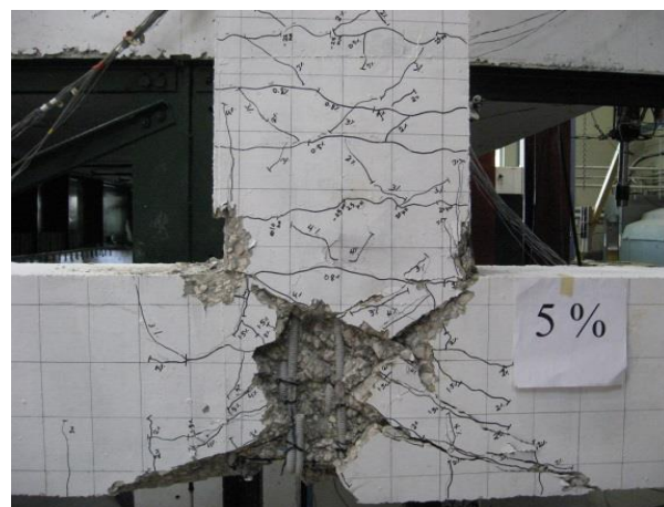
(h) Joint at Failure; zoom in
