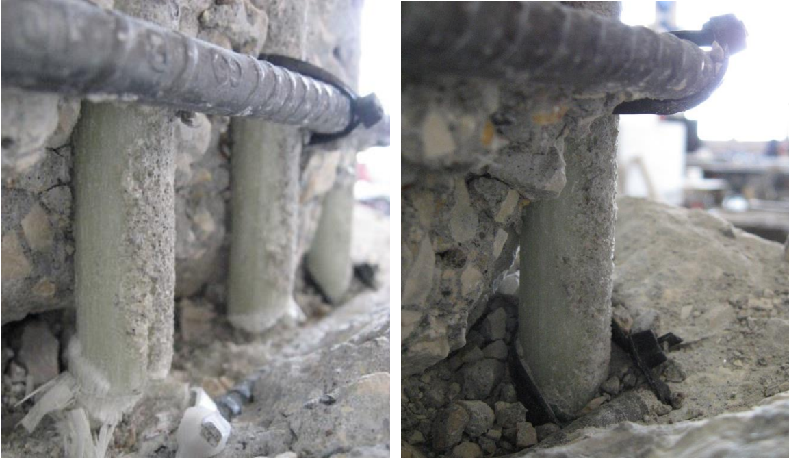
(a) Shearing-off in sand coating on the bars
