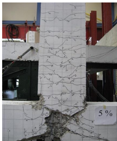
(g) 5.0% drift ratio; Failure
