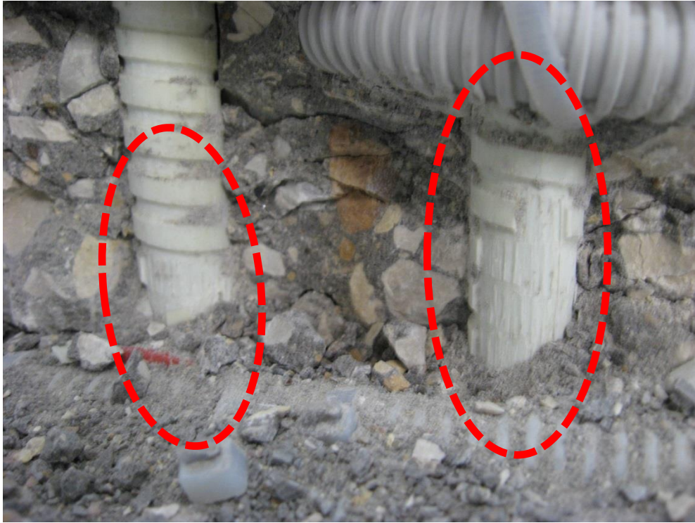
(b) Shear-off in bar ribs
