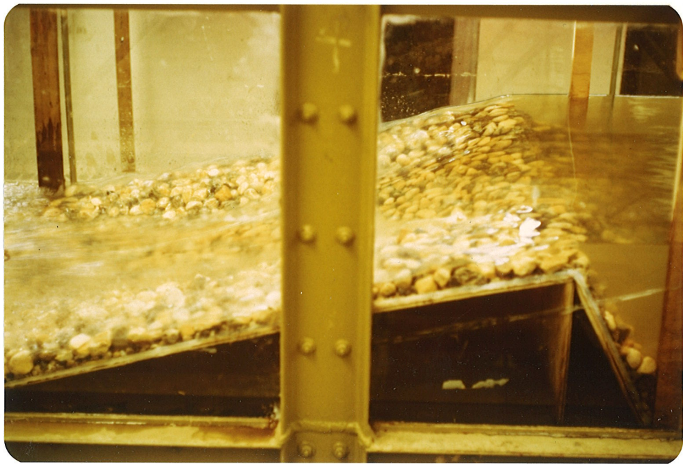
Plate 16 Side View - Roughened Top Layer Permeable Model at Maximum Discharge Tested ( d_{50} = 23 mm)
