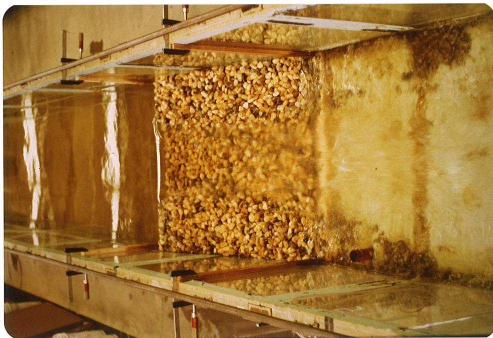
Plate 14 Roughened Top Layer Permeable Model at Design Discharge ( d_{50} = 23 mm)
