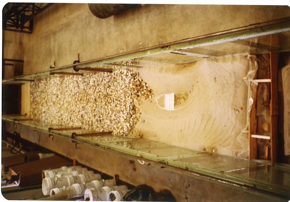
Plate 8 Silica Sand Bed Downstream of Model Following Testing
