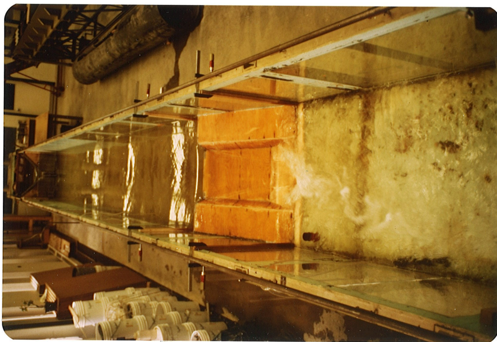
Plate 12 Smooth Impermeable Distorted Model at Design Discharge
