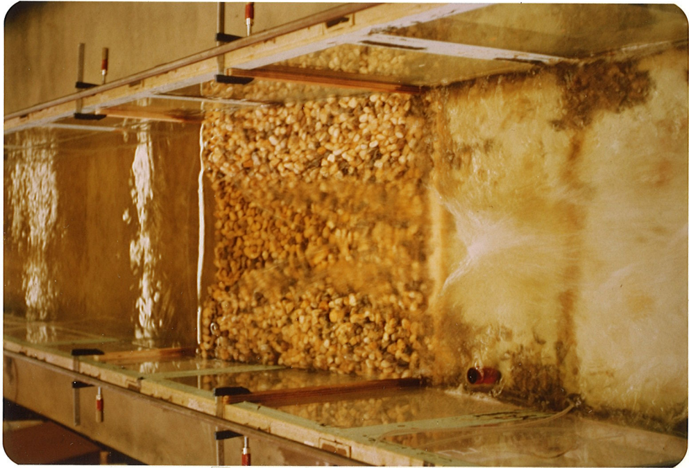
Plate 15 Roughened Top Layer Permeable Model at Maximum Discharge Tested ( d_{50} = 23 mm)
