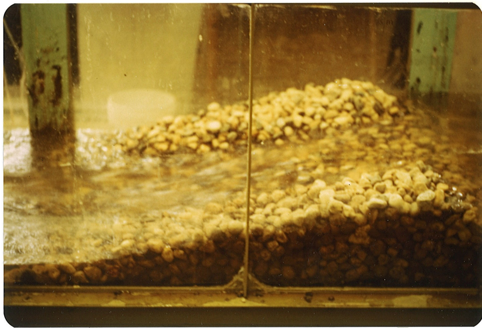
Plate 18 Side View - Completely Permeable Model at Design Discharge ( d_{50} = 23 mm)
