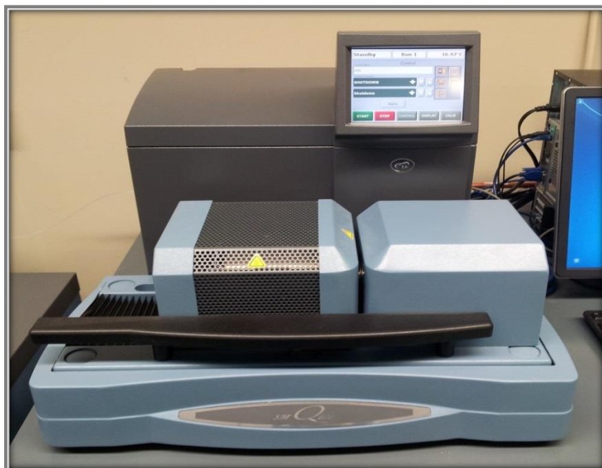
Figure 3.7: DSC instrument where the powder samples were mounted.
