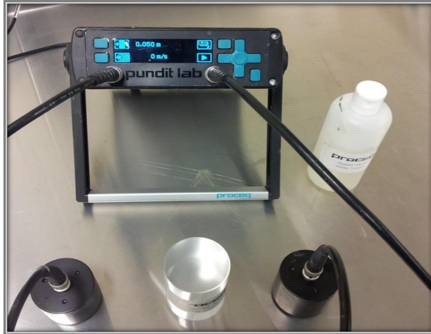
Figure 3.4: Ultrasonic Pulse Velocity (UPV) test apparatus used to determine the DME.
