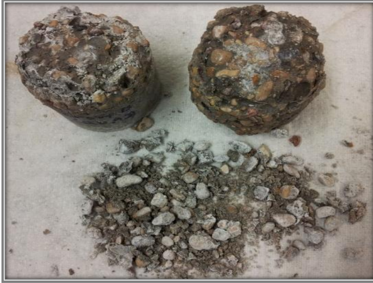
Figure 4.6: A specimen (75×150 mm) from GUA3-0.5 after breakage at 58 days.
