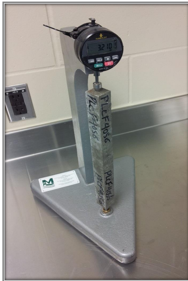
Figure 3.3: Length comparator utilized for determining the change in length of mortar bars.
