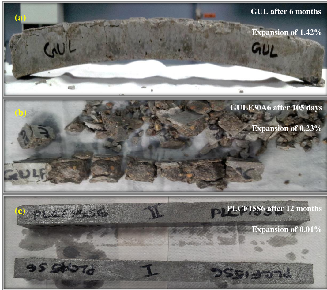
Figure 5.10: Visual features of mortar bars exposed to sodium sulfate solution at 5°C: (a) microcracks and expansion of a GUL specimen, (b) breakage of GULF30A6 specimens, and (c) intact PLCF15S6 specimens.
