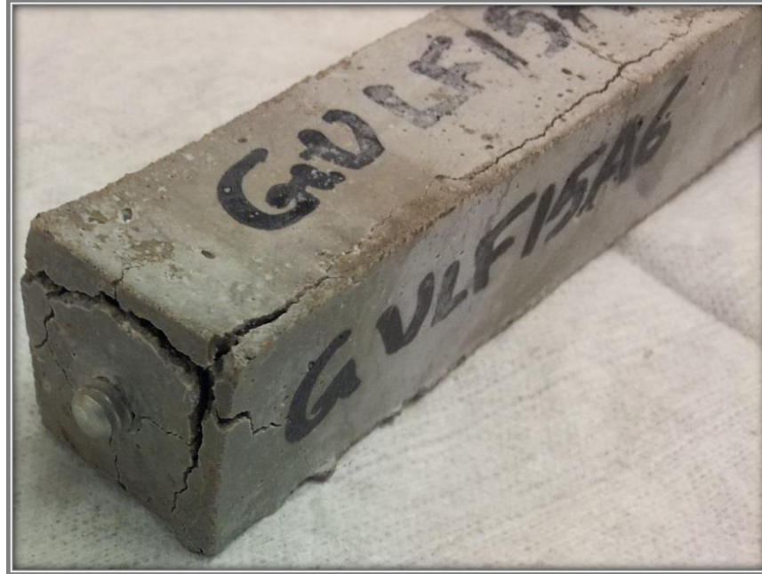
Figure 5.2: Cracks at the side and along the edge of GULF15A6 mortar bar (25×25×285 mm) after 120 days of exposure to conventional sulfate attack.
