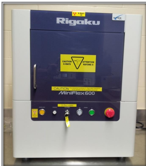
Figure 3.6: XRD instrument where the powder samples were mounted.
