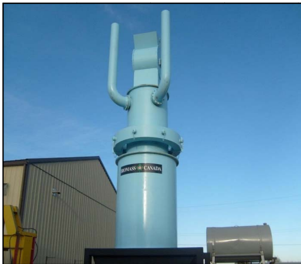
Photo 5-3: Second generation stratified catalytic downdraft gasification pilot plant of Biomass Canada, Edmonton, Alberta (Source: Mr. David Patterson).
