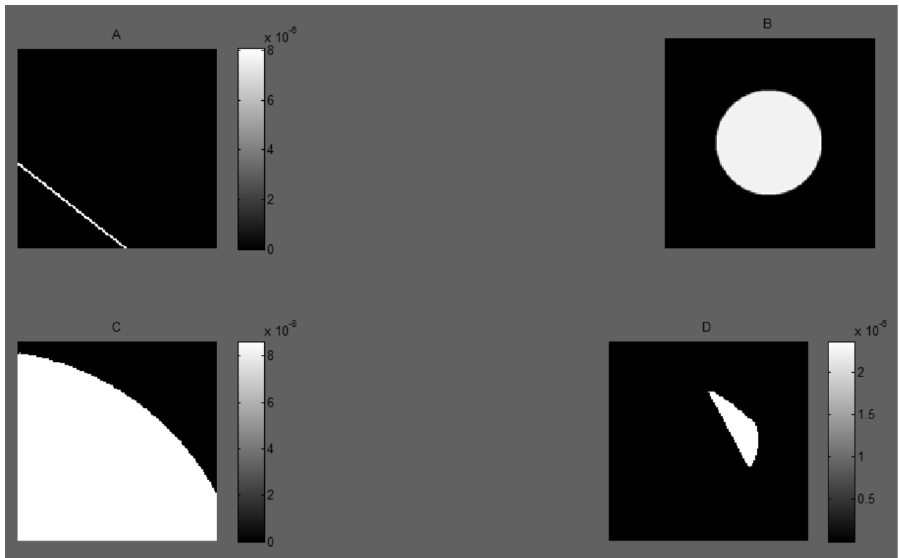
Figure 2-5. Example of probability images in different reconstruction techniques. (A) is a sample probability image (one row of the system matrix) for a scattered event when conventional list-mode method for system matrix generation was used, (B) shows the CT image of the cylindrical phantom, (C) shows the probability image when uniform projector/backprojector is applied but information regarding patient outline is not used, and (D) shows the same probability image as in (C), however, this time patient outline information is used.
