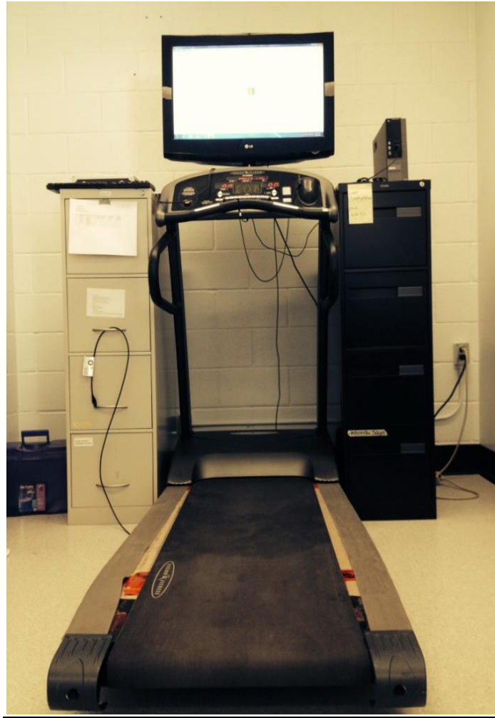
Figure 1: Force Sense Array mat placed under the walking belt of treadmill
