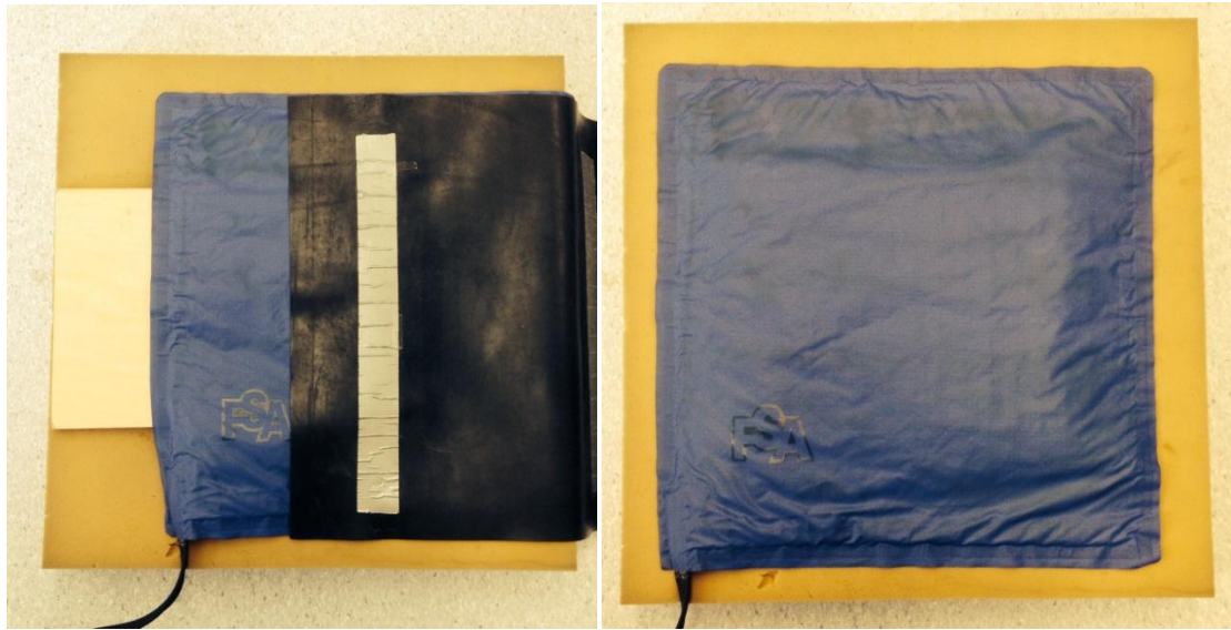
Figure 2: FSA mat used to collect CoP Excursions during standing task
