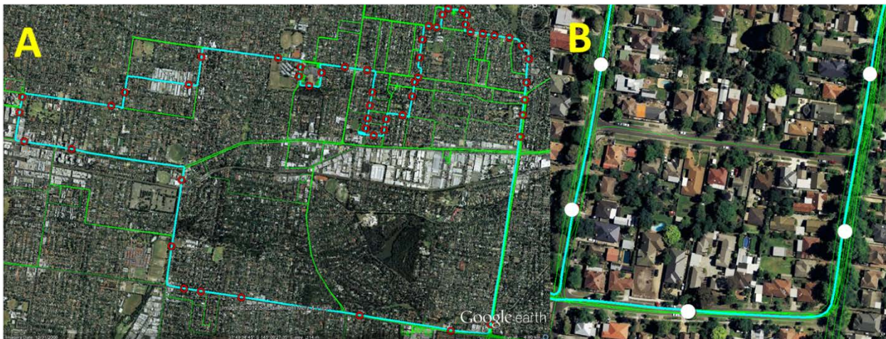
Figure 2. A) Trip locations visualized using Google Earth. The blue line denotes the entire driver observation schedule (DOS) trip, the green line shows all everyday driving trips, and the red circles identify locations where counts were taken. B) This is a closer view of A whereby the DOS route can be seen overlaid on multiple everyday trips. The white circles indicate locations where counts were taken.
