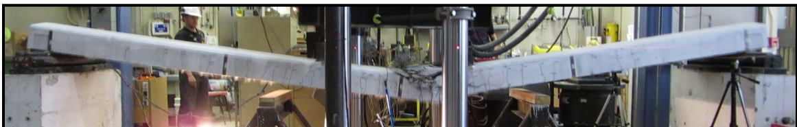
Figure 4-5 Slab F-0-3 (Compression Failure)
