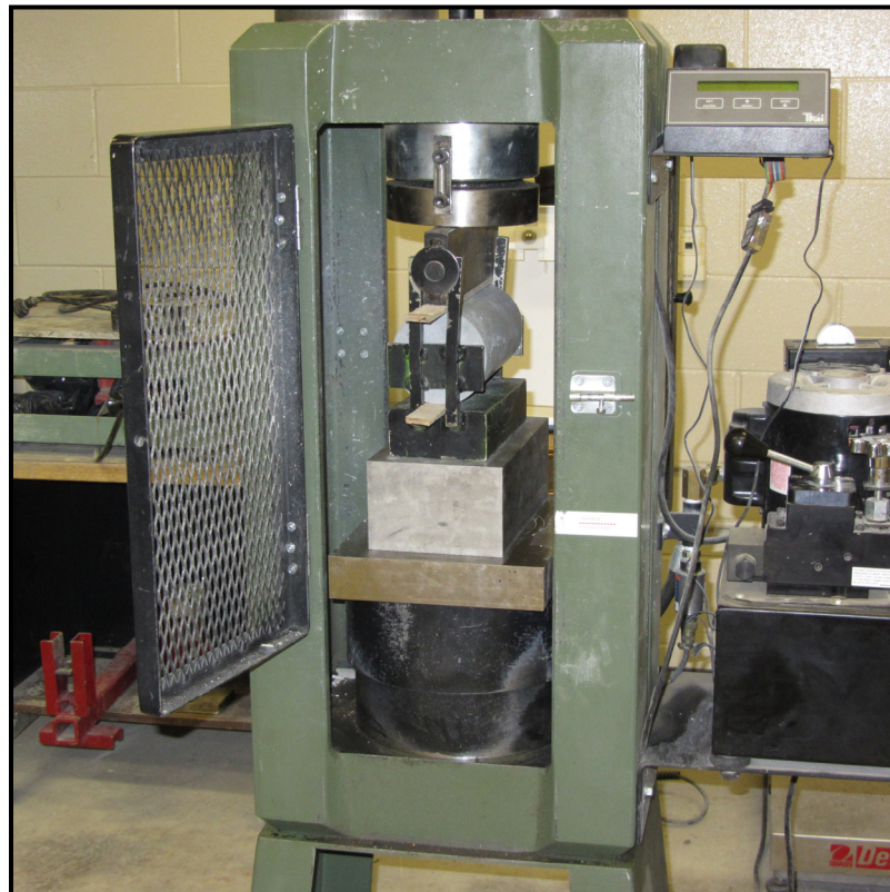
Figure 3-12 Split Cylinder Test Setup
