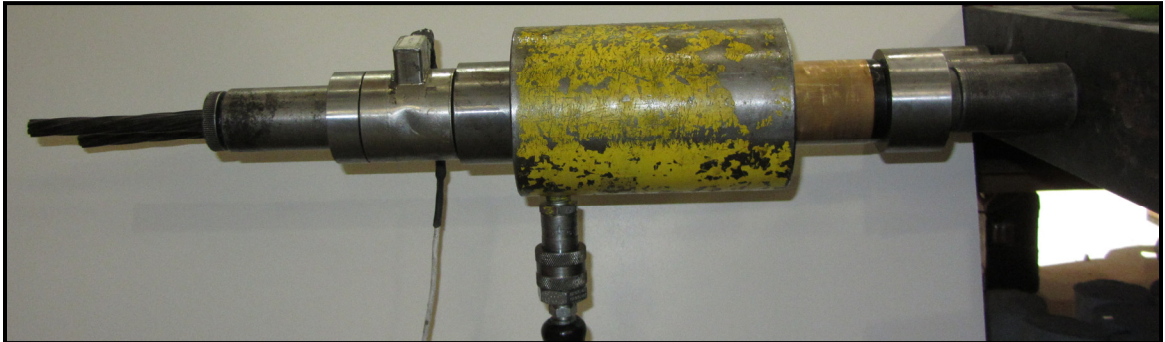
Figure 3-19 Hydraulic Jack and Load Cell Setup
