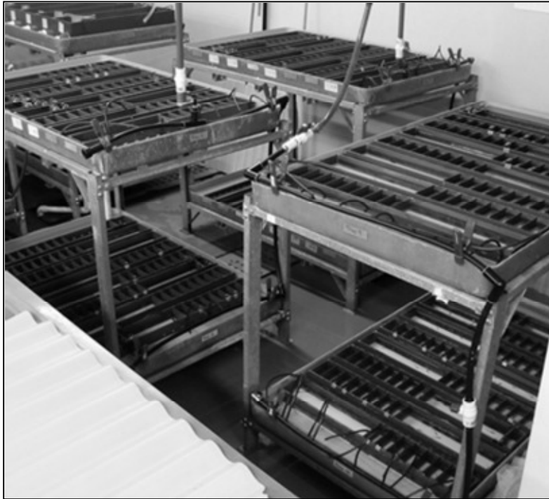
Figure 2.2 Laboratory set-up showing experimental tanks positioned in larger trays. Water was introduced at one end of the tray, passed through experimental tanks and exited a standpipe located at the opposite end.
