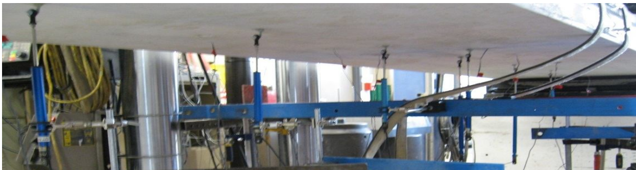
Figure 3.13: Instrumentation - LVDT Layout
