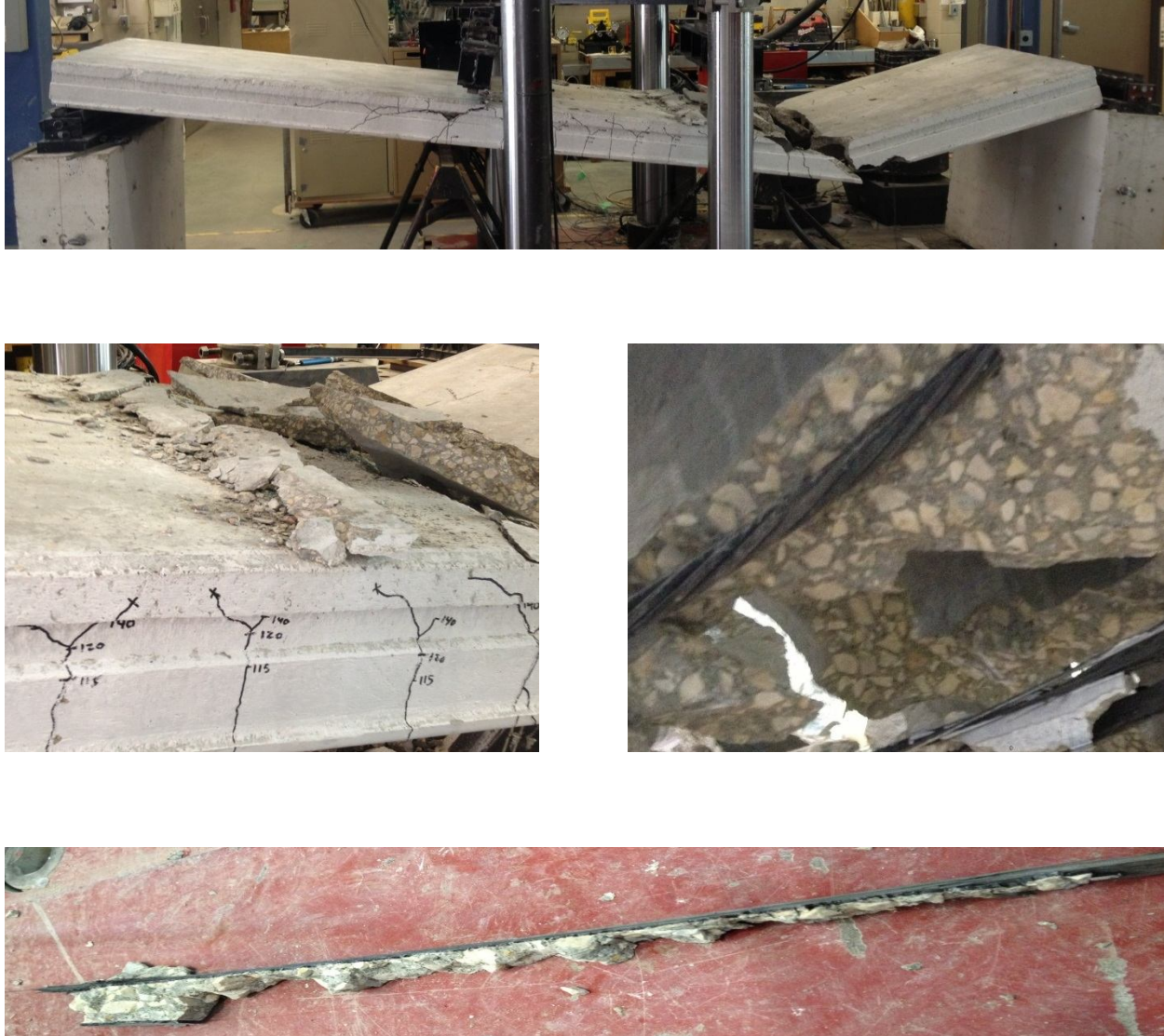
Figure G.7: I-2-S2-NO Mode of Failure
