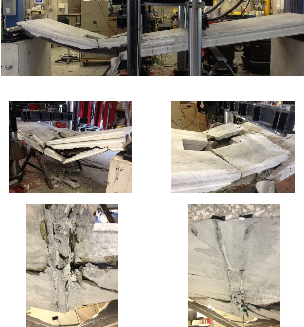
Figure G.11: III-1-S2-SO Specimen at Failure
