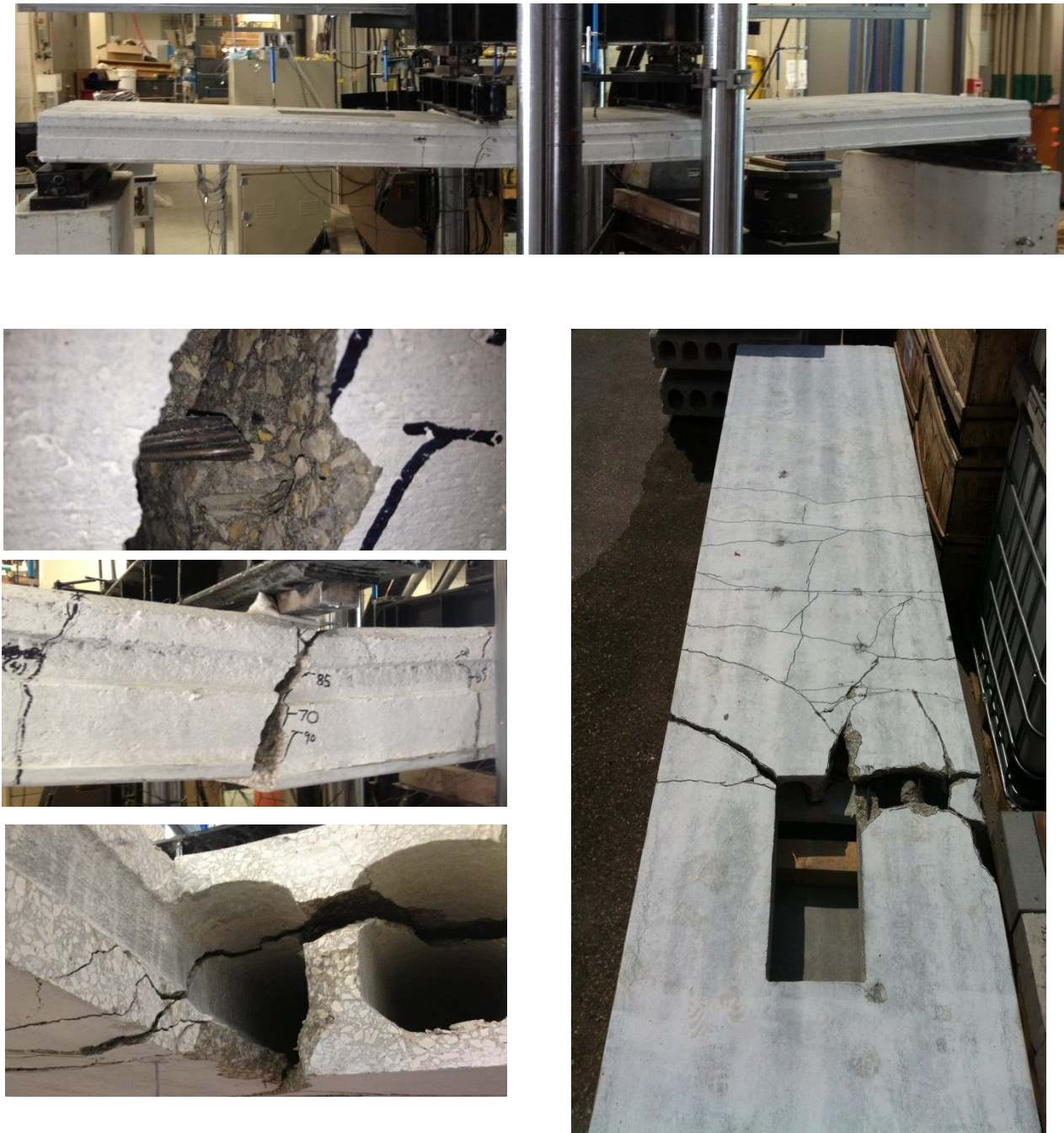
Figure G.9: II-1-S0-SO Specimen at Failure
