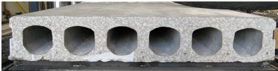
Figure 3.2: Typical Hollow-Core Slab Cross Section
