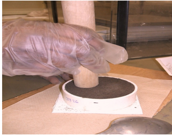
Figure 3.1 Soil container after the incorporation of designated amendment and moisture (WFPS) being packed at bulk density of 1.2 \text{ gcm}^{-3}
