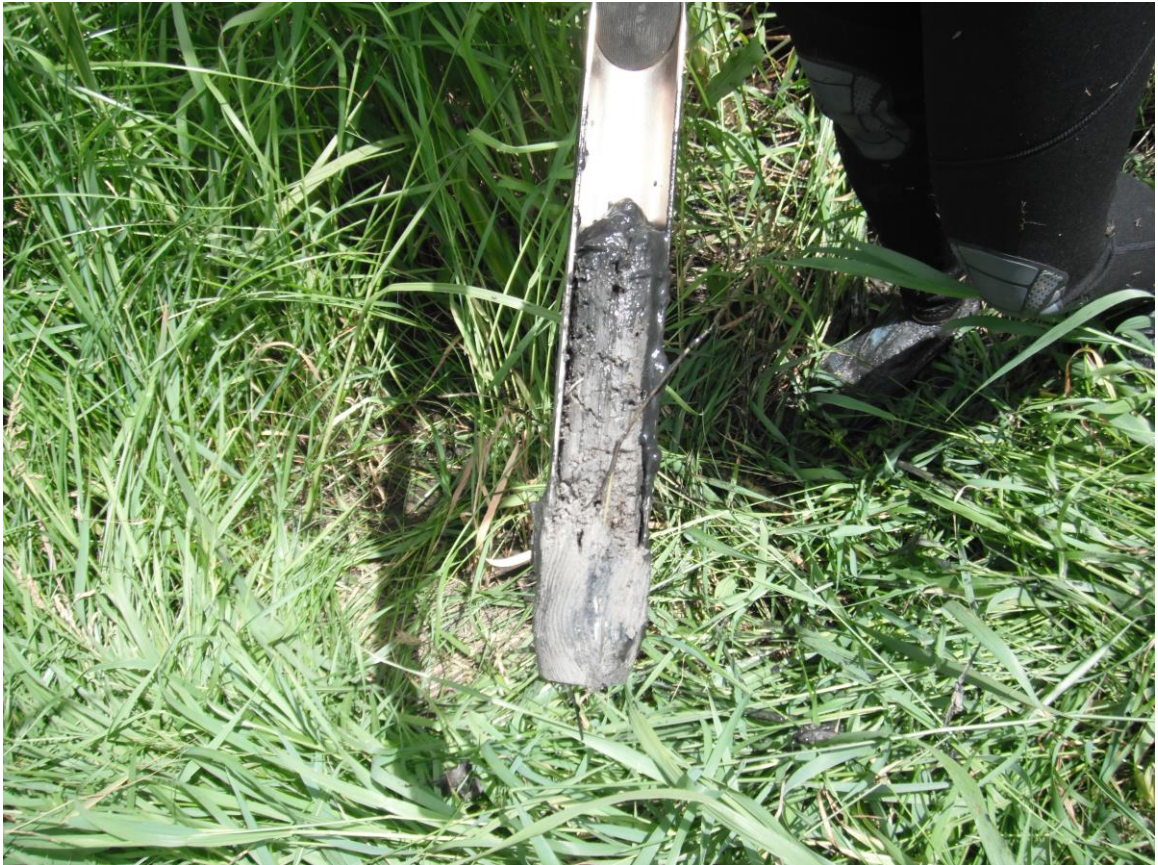
Fig. 3.3 Soil corer used to extract 10 cm long sediment cores from cattail pothole and ditch marshes in southwestern Manitoba and southeastern Saskatchewan, 2011
