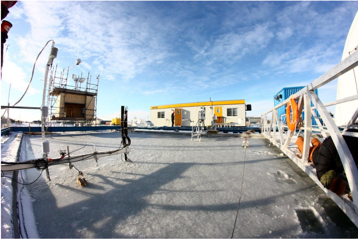
Figure A3.1: Photo of the SERF site at the University of Manitoba, taken in January 2013. The experimental sea ice was approximately 7 cm thick at this time.
