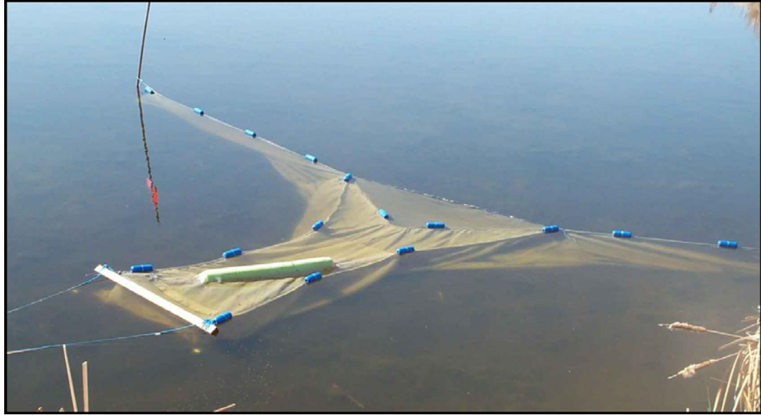
Figure 3-2. Beamish trap with a modified 15 cm opening for use in shallow water. Traps were set in 10 study ponds in Delta Marsh between early June and late August, 2001 and 2002.
