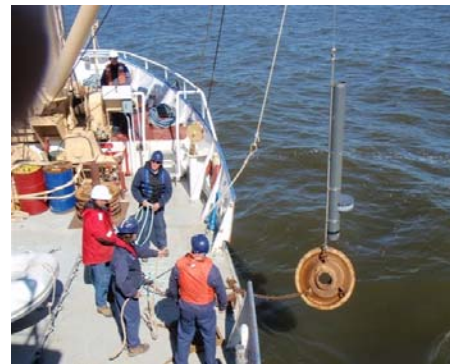
Sequential sediment trap is deployed from the deck of the MV Namao. Photo Credit: Todd Breedon. © Environment Canada 2009
