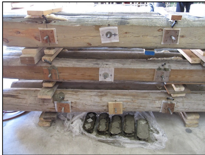
Figure 3-12. Additional grout cores at quarter span.
