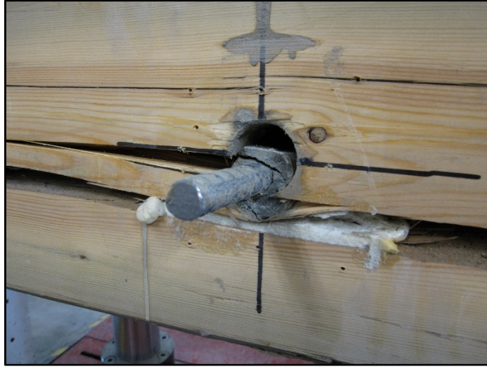
Figure 4-3. Horizontal shear failure around grout core.
