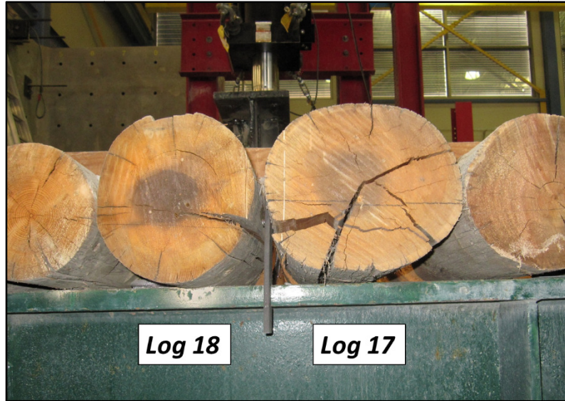
Figure 4-13. Horizontal shear failure of Log #17.
