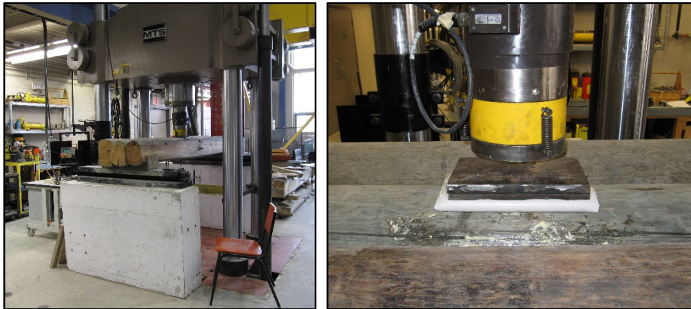
Figure 3-11. Static test setup and load plate at middle log.
