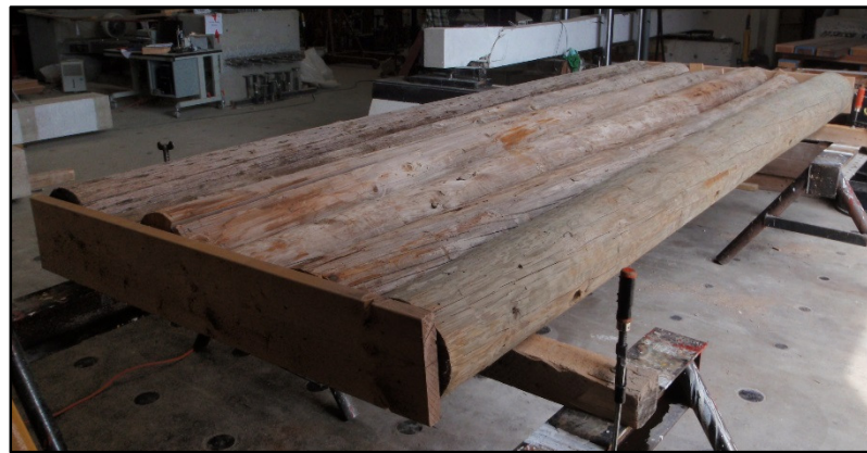
Figure 3-14. Full-scale panels with end boards.
