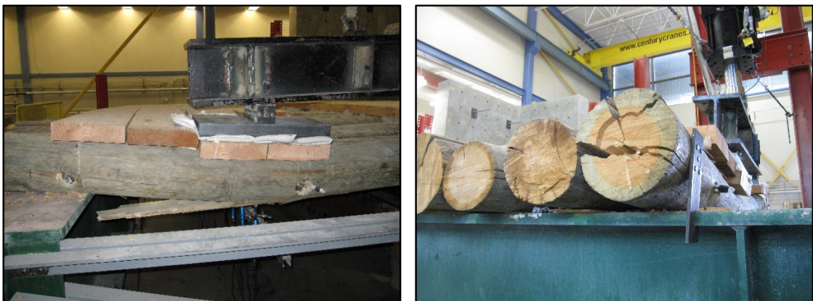
Figure 4-7. Tension and horizontal shear failure of outer log.
