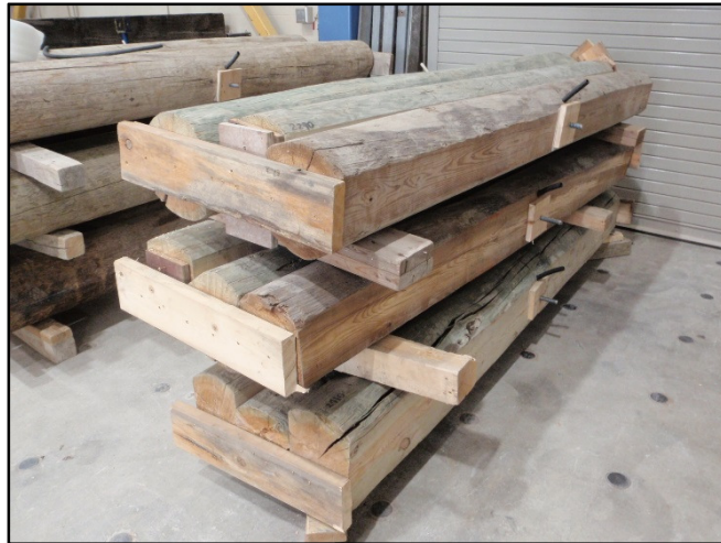
Figure 3-5. Timber boards holding planed logs in place.
