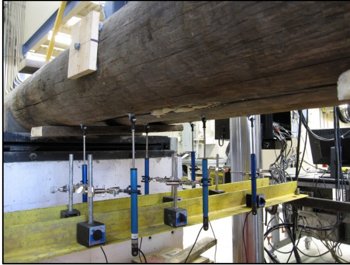
b) Placement of LVDTs under each log
