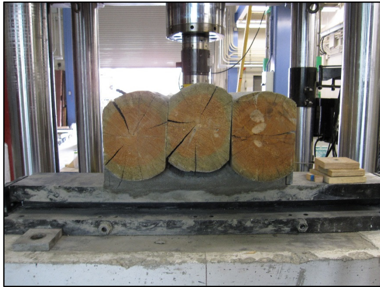
Figure 3-10. Grout placed underneath logs at supports in small-scale assemblies.
