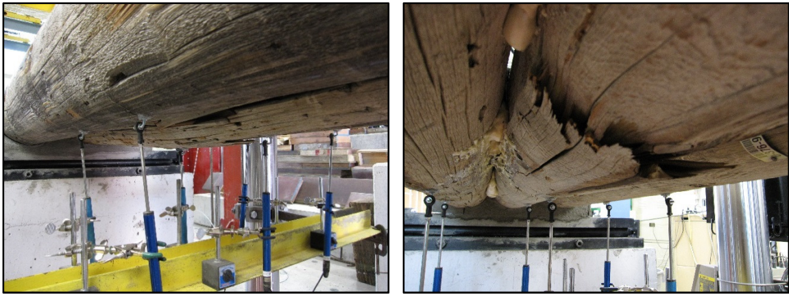
Figure 4-4. Tension failure of round log panels.
