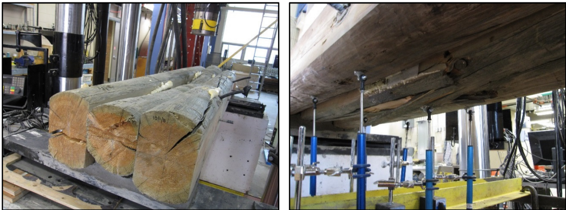
Figure 4-2. Deformation and tension failure in planed log panels.
