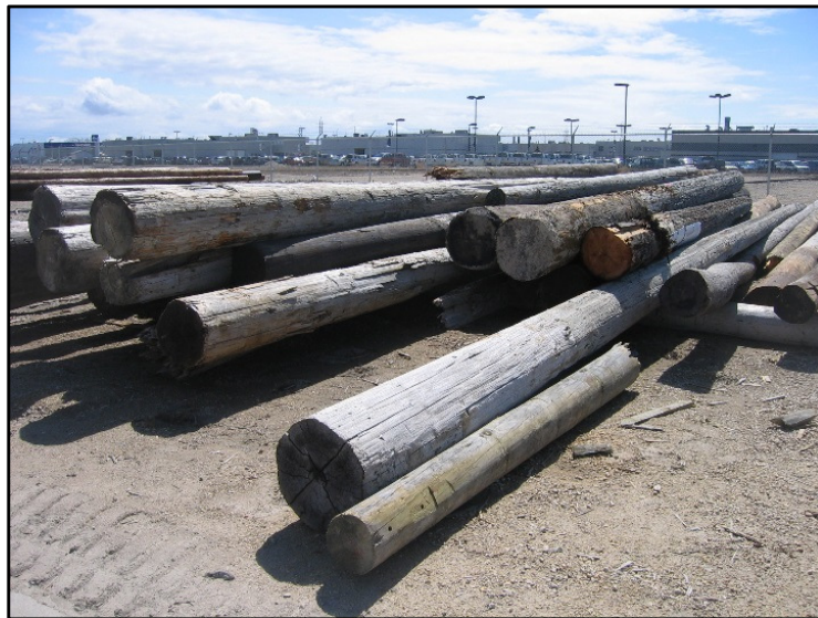
Figure 3-2. Timber logs for deck panels.
