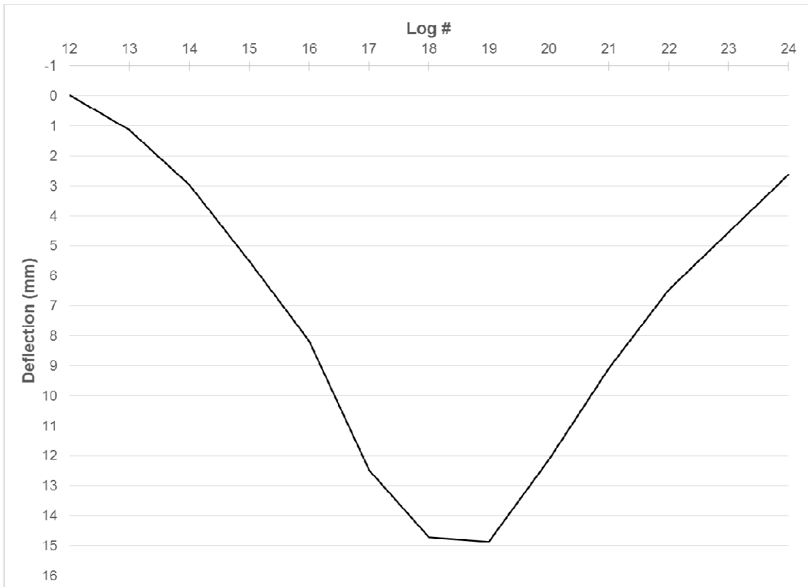
Figure 5.3. Deflection measurements across the logs at 300 kN.
