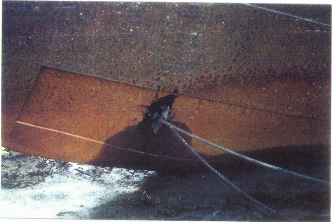
Figure 4b. Cable attachment point on port bow of the Graham Bell.
