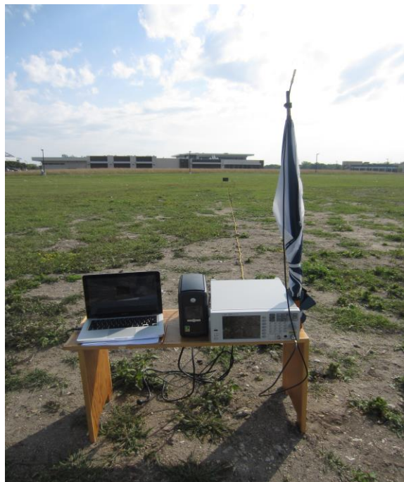
Fig. 30. Outdoor measurement setup at receiver end.
