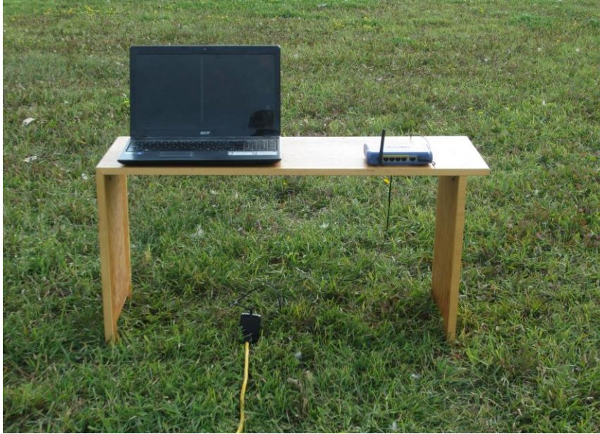
Fig. 29. Outdoor measurement setup at transmitter end.
