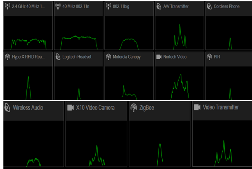
Fig. 32. Matching signatures of the captured signal at the experiment location.
