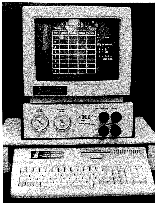
FIGURE II-2: Flexercell Strain Unit R . The vacuum gauge on the far left of the control module measures the amount and stability of the system vacuum. The Flexercell vacuum gauge (second to the left) measures the vacuum applied to the silicone membranes of the culture dishes.
