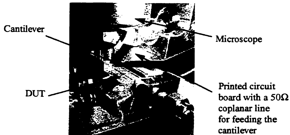
Figure 3.11: A zoomed view of figure 3.10 showing the cantilever and DUT.
