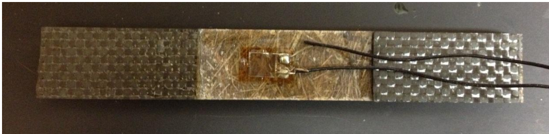
Figure 4.3. The test coupon with strain gauge
