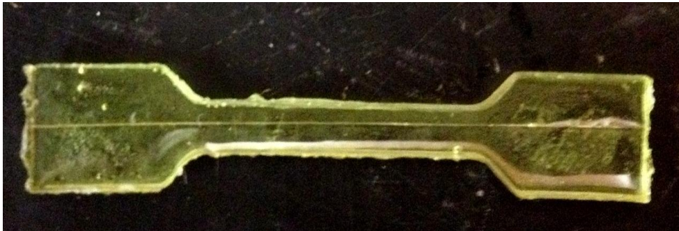
Figure 4.13. Single fiber fragmentation test specimen
