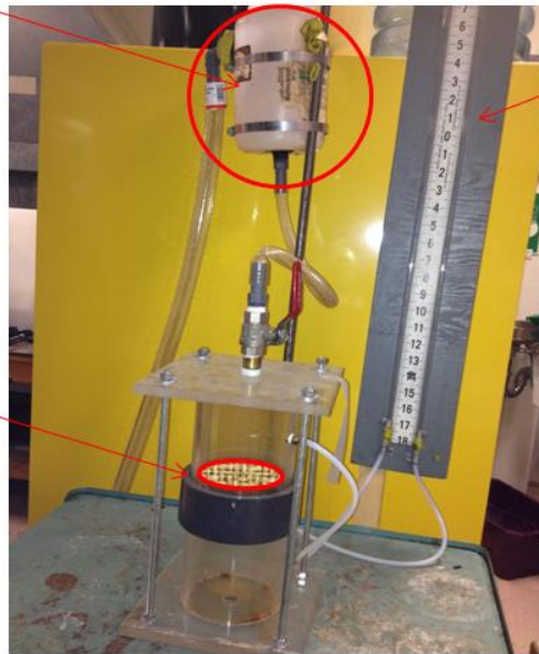
Figure 4.8. Transverse Permeability test setup
