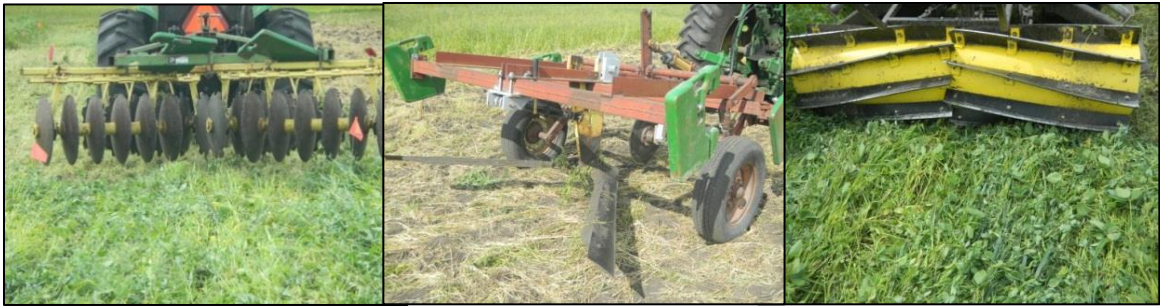
Figure 1. Implements used for management of the green manure crops at Carman (L-R): disc, wide blade cultivator (Noble blade), blade roller.
