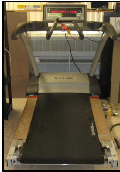
Figure 1: Treadmill instrumented with a force sensory array mat
