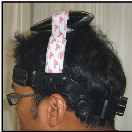
Figure 4: Gyration Air mouse mounted on a helmet with Velcro
