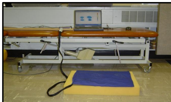
Figure 2: Standing FSA mat used to record COP excursions.
