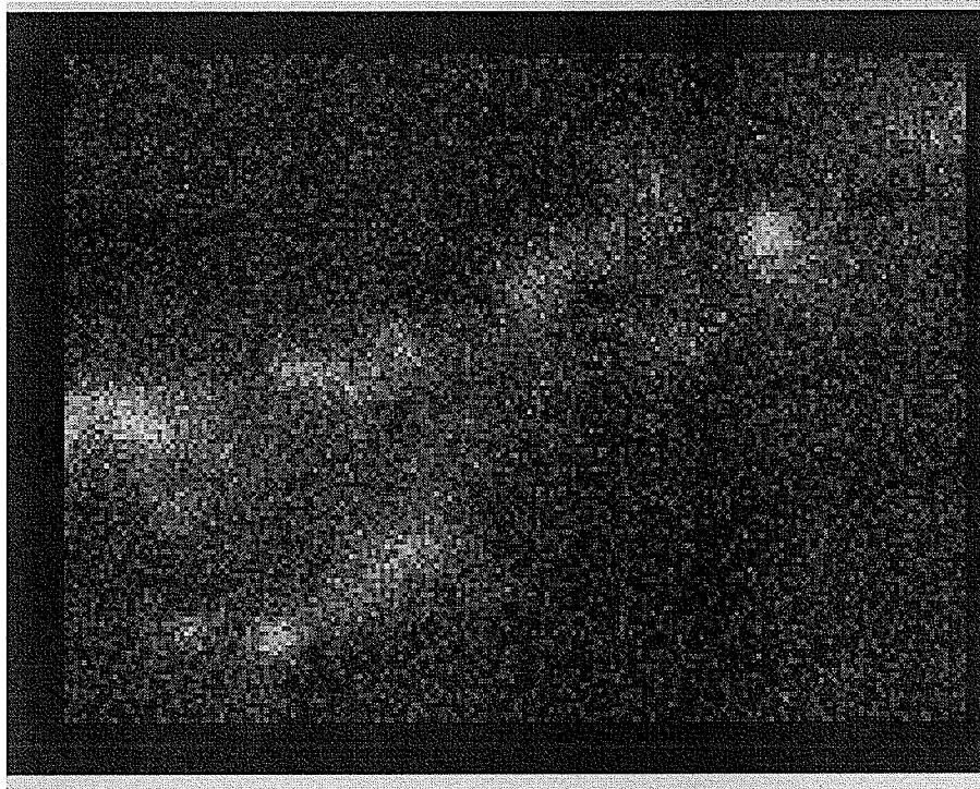
Fig. 4.40 (a) Resolidified products at the crack edges (b) SEM/EDS X-ray mapping of Nb around the crack showing enrichment in the resolidified products
