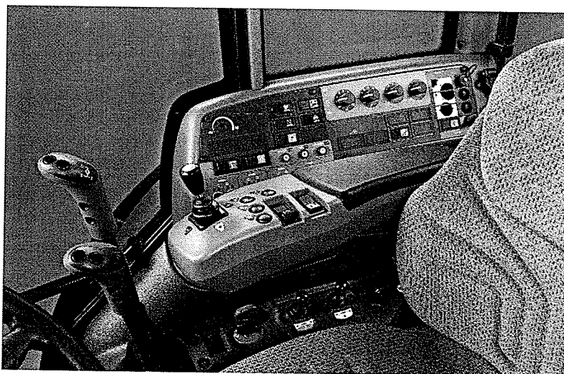
Figure 2.3 Control panel of a tractor based on hand-levers, joysticks, buttons, rocker switches and knobs (Source: Valtra tractors 2005)
