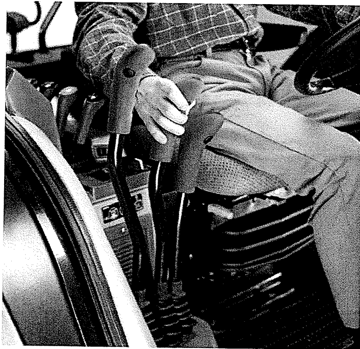
Figure 2.5 The sequence of use principle based on three hand-levers with declining height
