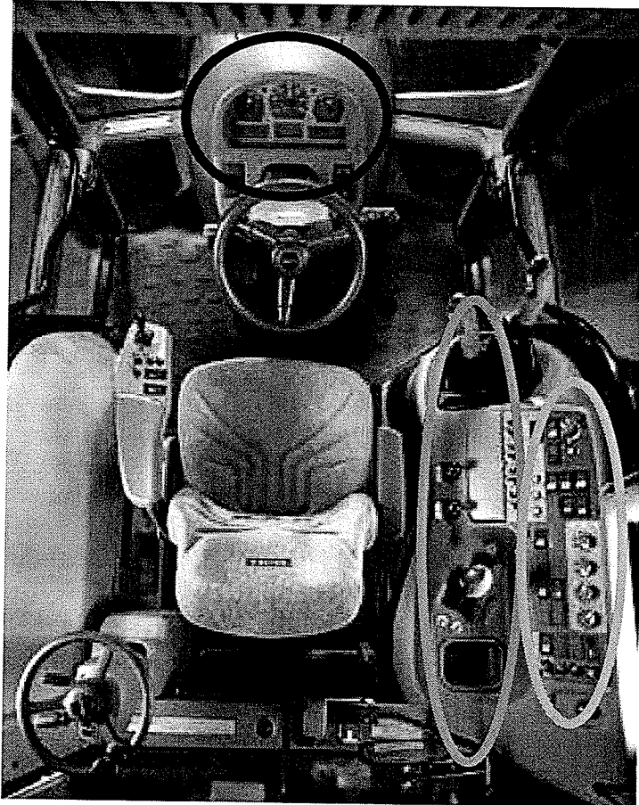
Figure 2.1 The three basic zones of controls in a tractor cab (Source: Valtra tractors 2005 )
