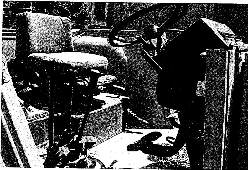
Figure 2.2 Control panel of a tractor based mainly on hand-levers
