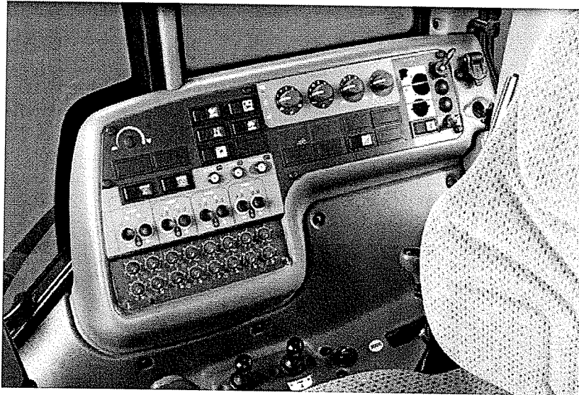
Figure 2.4 Control panel of a tractor based on joysticks, buttons, knobs and rocker switches (Source: Valtra tractors 2005 )
