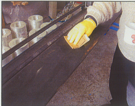
Figure 4-7 Applying releasing agent on the surface of the mandrel
