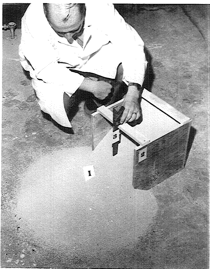
Figure 14. Test apparatus for angle of repose showing: 1. fertilizer sample, 2. test box and, 3. combination square placed to measure S distance.
