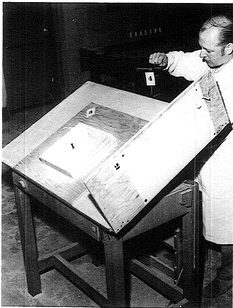
Figure 13. Test apparatus for coefficient of friction showing: 1. fertilizer sample in frame, 2. protractor and plumb bob, 3. sample of plywood fastened to table top and, 4. bar clamp for raising table top.
