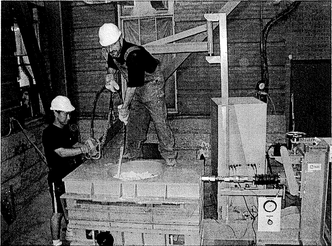
Figure 3.7 Densification of rockfill materials in large direct shear box
