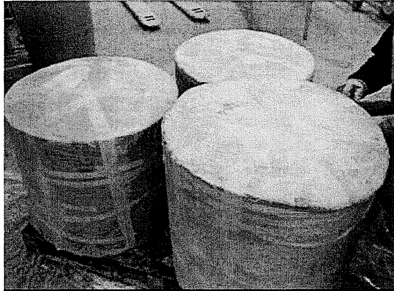
Figure 3.8 Waxing and rapping the undisturbed clay samples
