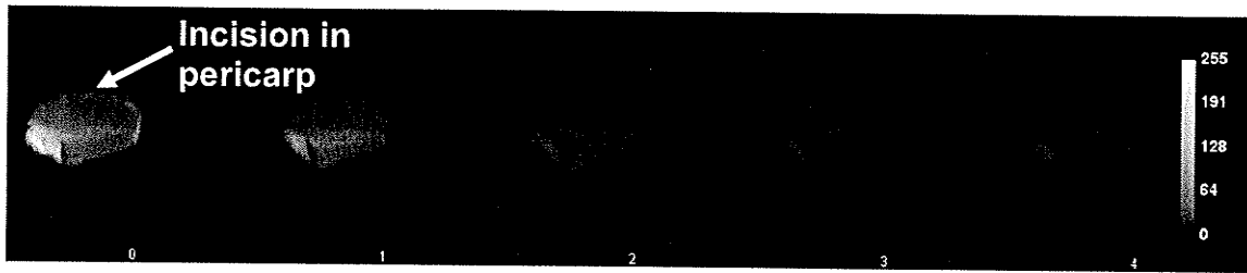
Figure 4.4a Magnetic resonance images of a mechanically scarified wheat kernel during drying at every hour. Drying conditions: temperature, 40°C; drying time, 4 h. Numbers at the bottom of the images indicate the time, in hours, from the beginning of drying.
