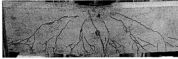
Figure 5.22: Crack Pattern of Control Specimen #2
