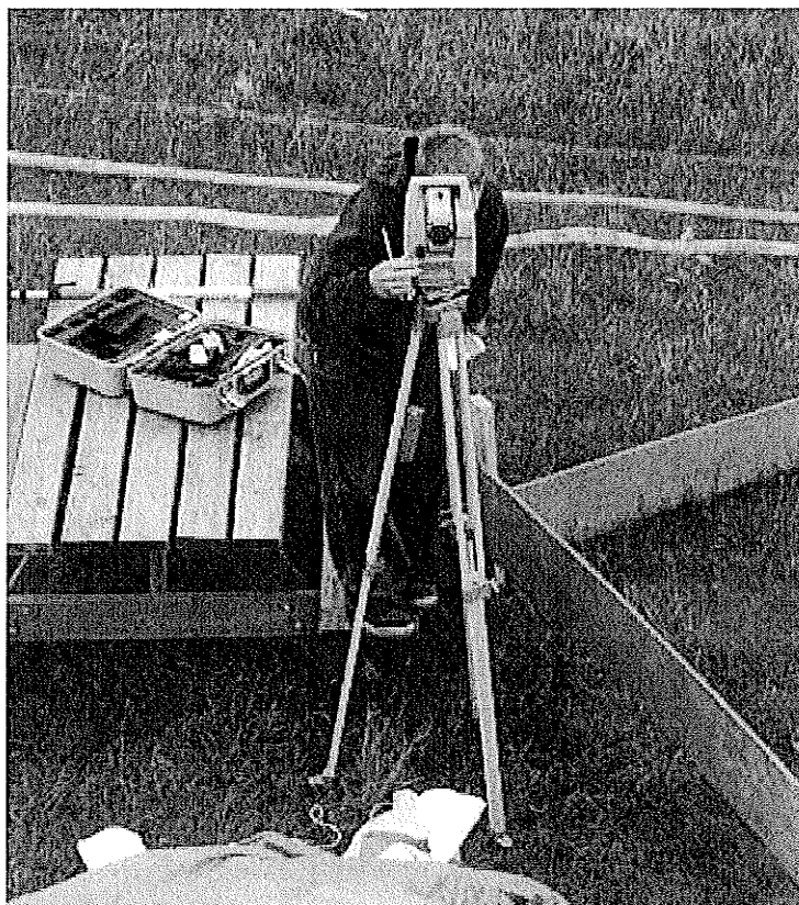
Figure 4.14 – Total Station being used to Survey Points on Sandbag Dike.
