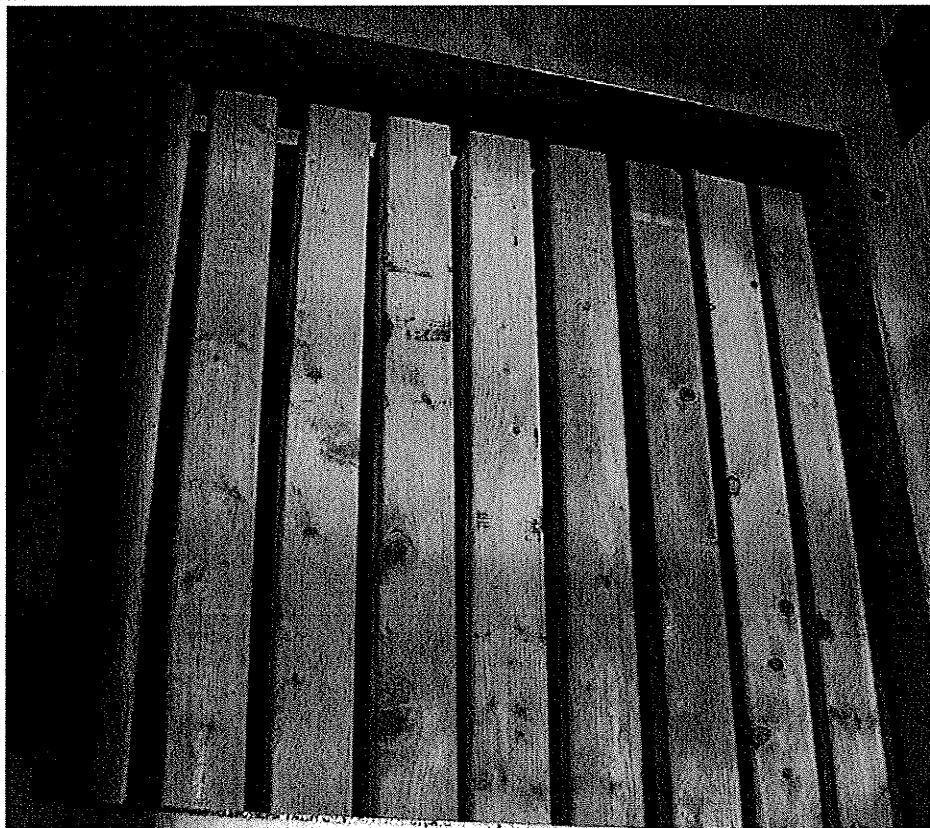
Figure 3.10 – Crib Support Material in Bottom of Large-scale Direct Shear Apparatus.
