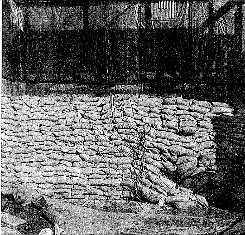
Figure 5.42 – Dike C3 Final Deformed Shape, Front View.
