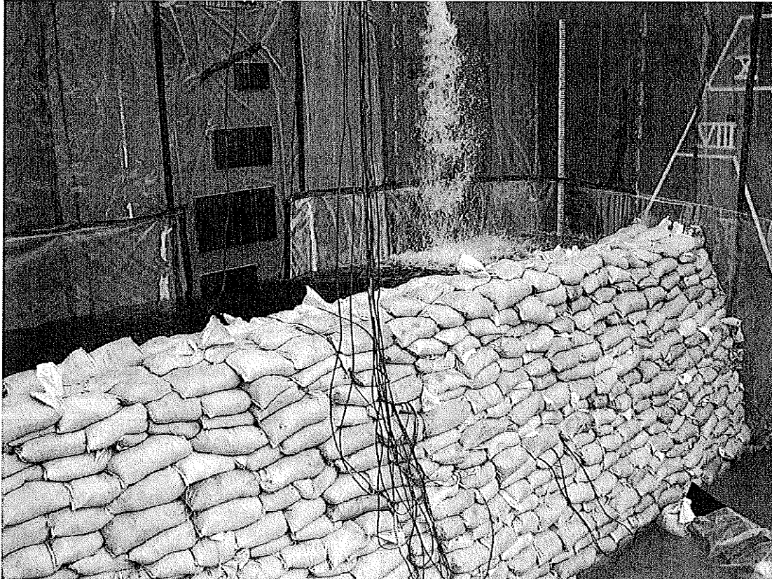
Figure 5.40 – Dike C1 at Above Design Loading, View to the East.
