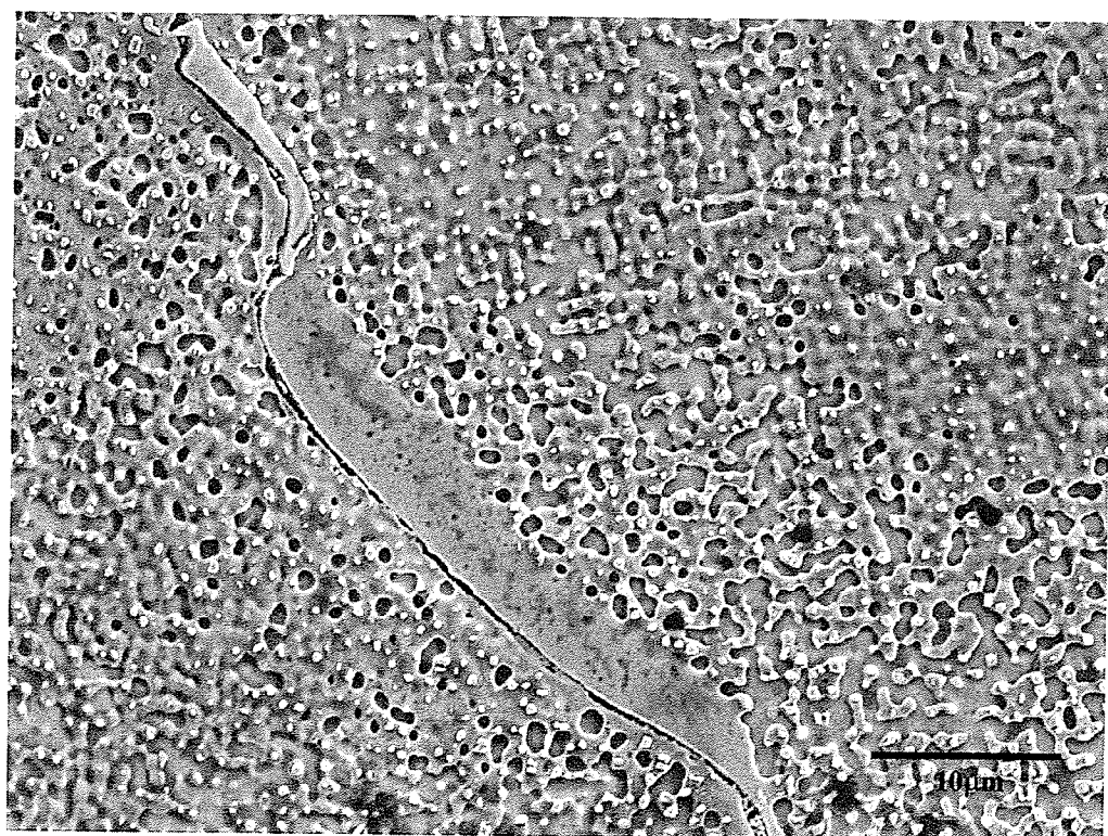
Figure 4.48: ST Gleble simulated HAZ at 1165°C for 4s
