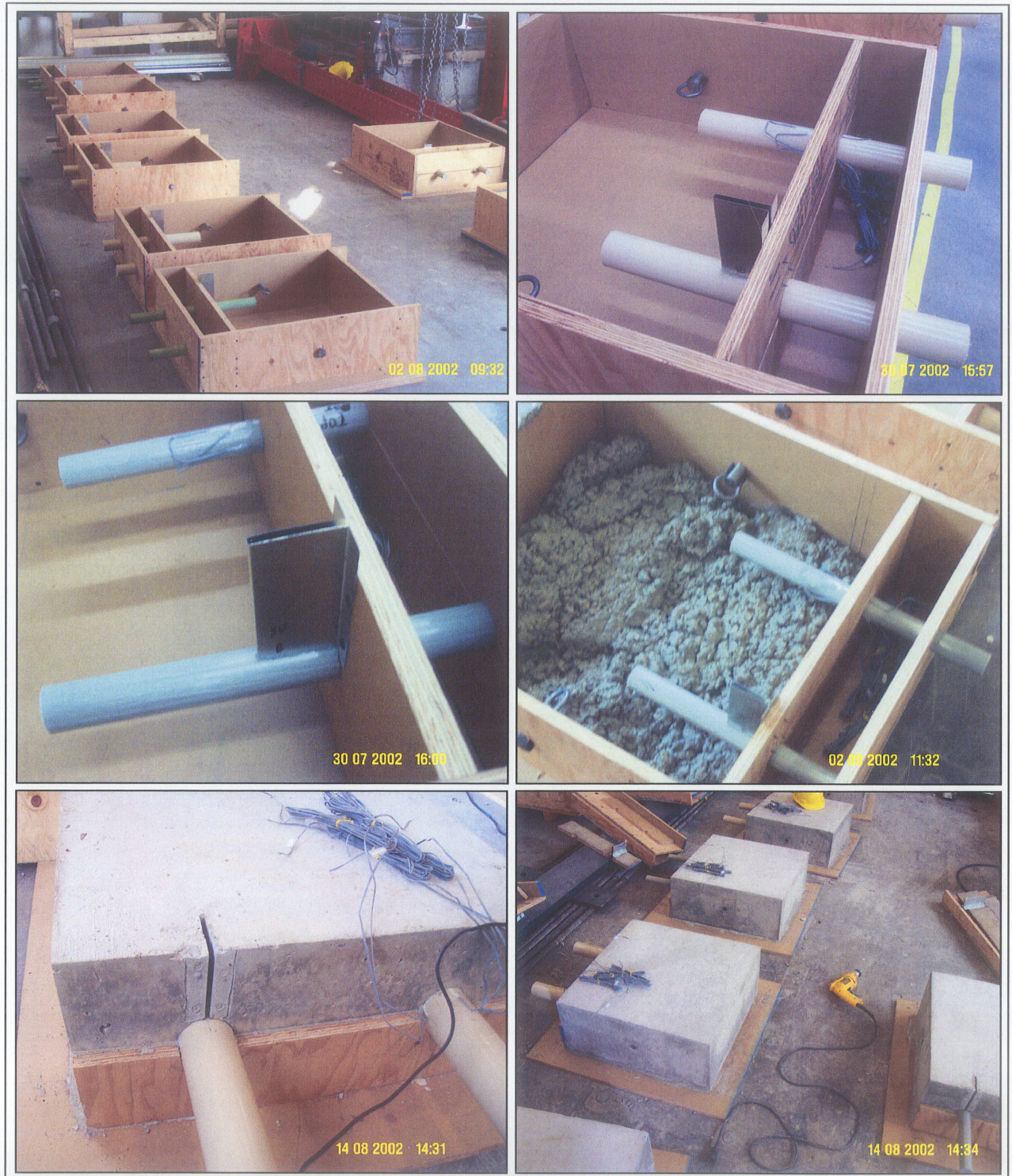
Figure 4.6: Fabrication of the Test Specimens
