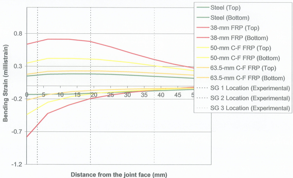
Figure 6.9: Axial strain in dowels due to bending at service load (FEM Results)
