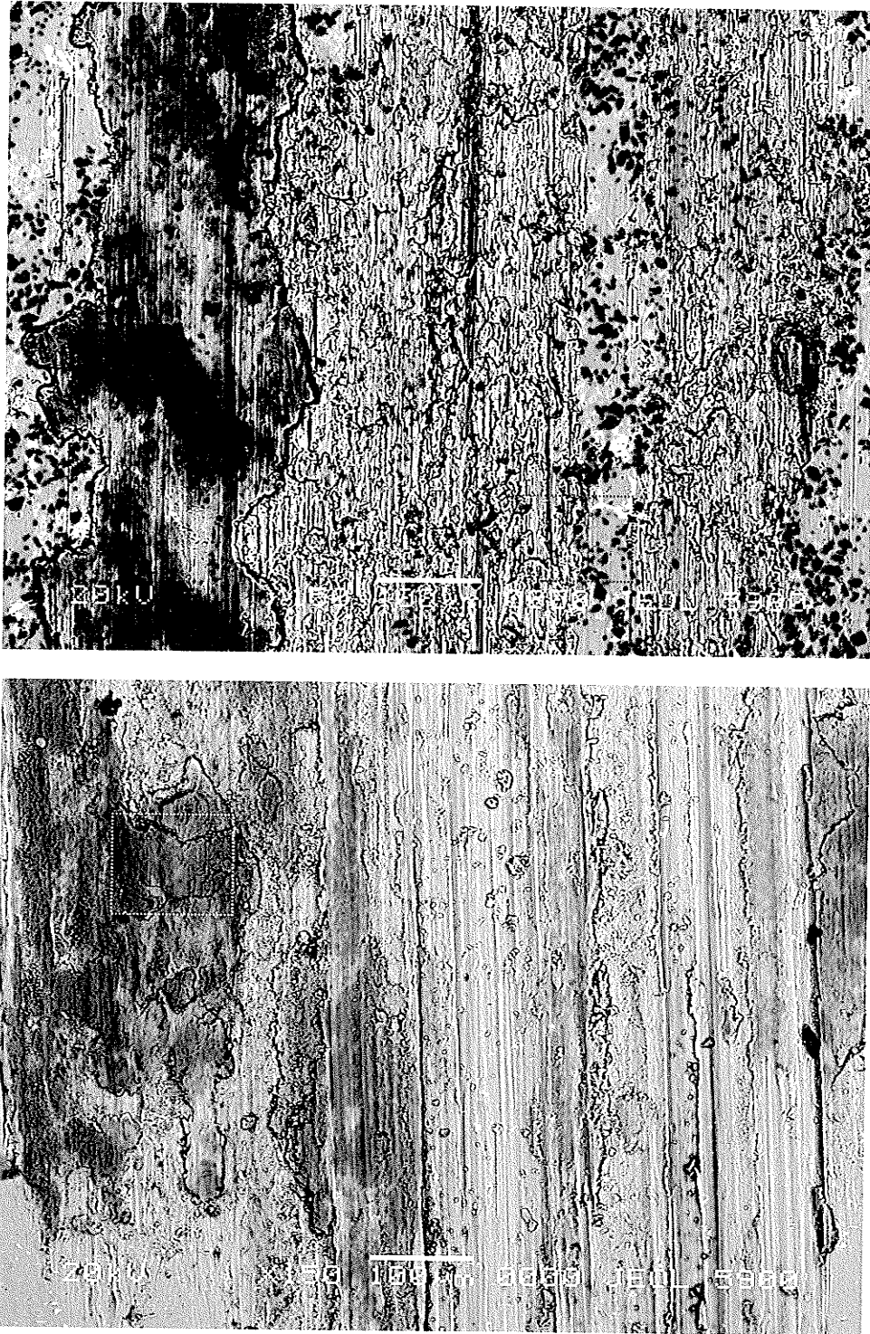
Figure 4.43 Al-6061 (BOTTOM) against the composite (TOP) 10m, 2N. Two distinct regions of SML formation are observed. On the left transfer of the Al-Si composite matrix caused a highly oxidized and smeared surface including crushed SiC. On the right transfer and back transfer of the Al-6061 matrix has caused a SML of the deformed matrix alloys overtop the reinforced composite surface.
