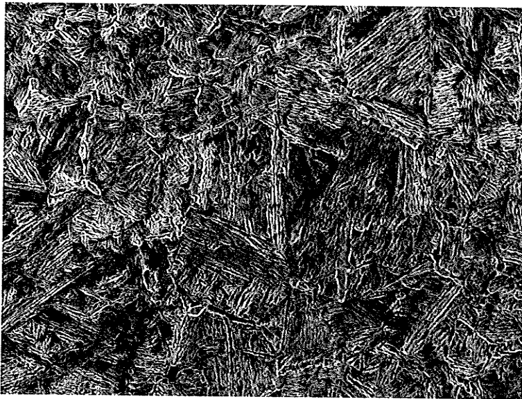
Figure 4.114 Center of as received 52100 ball bearing, 400x
